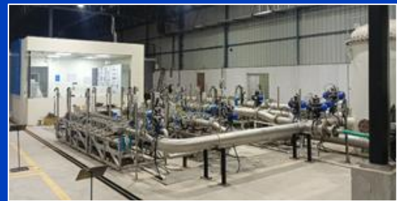
Figure 3. Calibration of magnetic flowmeters of sizes DN15 to DN300.
