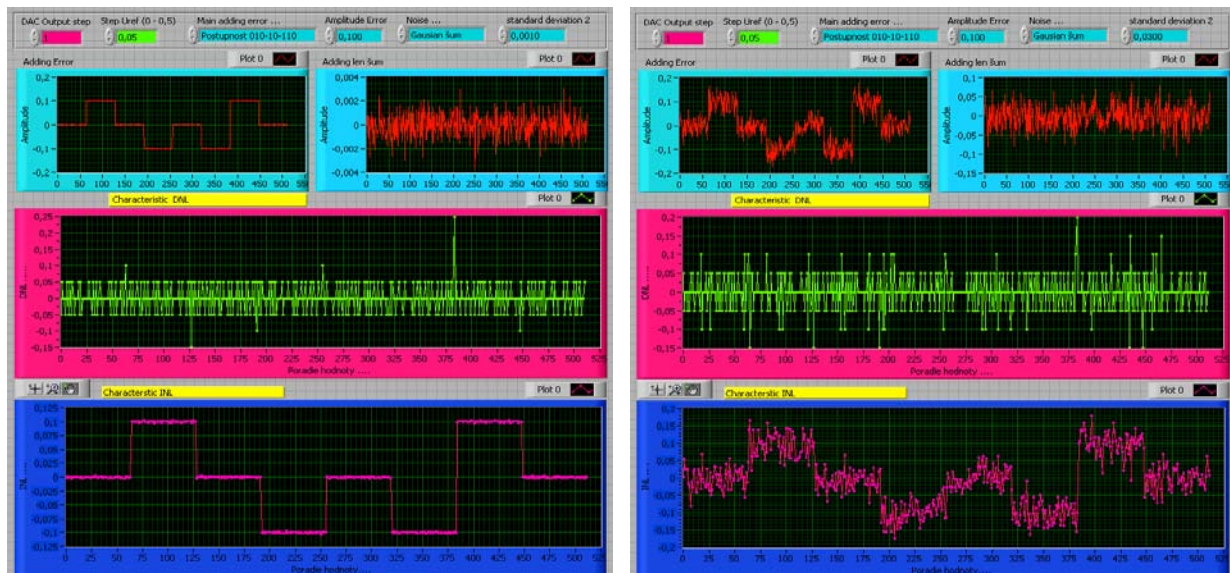
Figure 2. Simulation of precise time difference measurement for a 9-bit resolution DAC without noise (on left-hand side) and with noise (on right-hand side) in development environment
