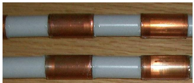
Fig. 4. Divided electrodes for the free water level measurement using simple two terminals experiment arrangement.
