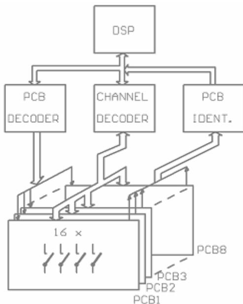
Fig. 5. Principal block diagram of the channel multiplexer.
