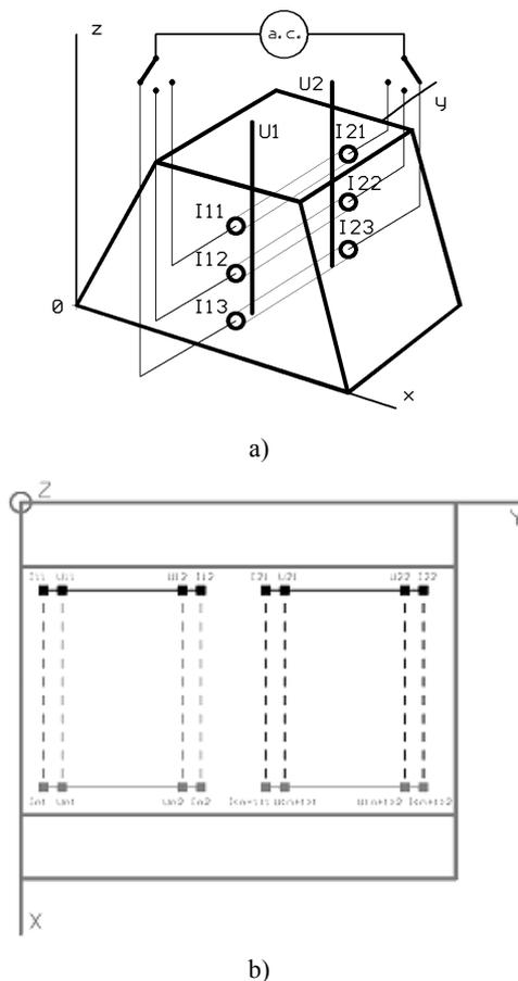
Fig. 2. The use of divided current electrodes makes possible to sample the dike space in  $z$  – direction (a), and higher density of electrodes in  $y$  – direction allows for the sampling of the space in  $y$  – coordinate.
