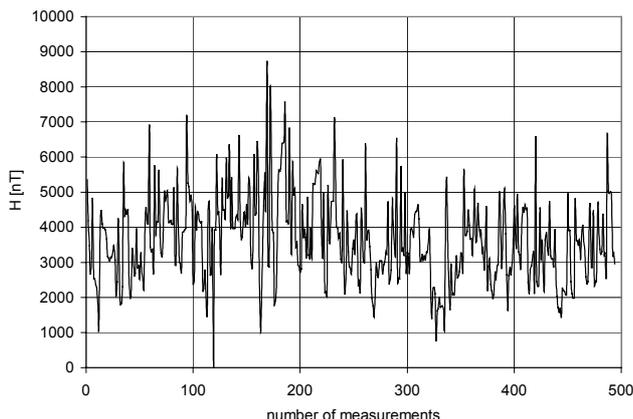
Fig. 1. The graph of magnetic field intensity changes in time in room no 4, for the measurements registered every 0.5 [s] and the number of 493-sample registration
