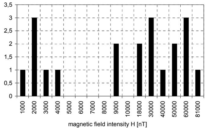
Fig. 6. The histogram of magnetic field intensity changes in time in the neighbourhood of hardening furnaces, for the measurements registered every 0.5 [s] and the number of 493-sample registration
