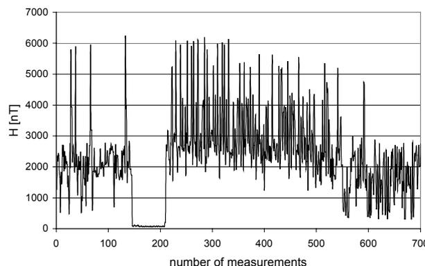
Fig. 5. The graph showing the changes in magnetic field intensity in time together with the registered change of the field to the value of the background (production break)
