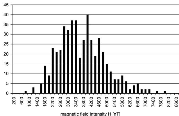
Fig. 4. The histogram of magnetic field intensity changes in time in room no 4, for the measurements registered every 0.5 [s] and the number of 493-sample registration
