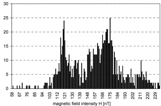
Fig. 6. The histogram of magnetic field intensity changes in time in room no 2, for the measurements registered every 0.5 [s] and the number of 493-sample registration (I measurements series)
