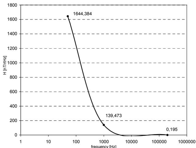
Fig. 2. Magnetic field spectrum – an assessment on the basis of maximal values of magnetic field intensities for the results obtained in all measurement bands
