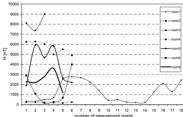
Fig. 3. Magnetic field intensity in the band from 5 Hz to 400 kHz in the selected rooms
