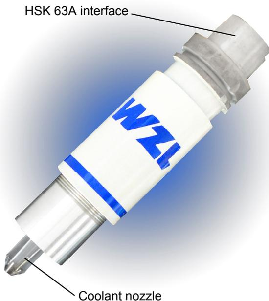
Fig. 10. WZL Ultrasonic sensor tool
