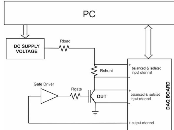
Fig. 1. Measurement system for static characteristics.
