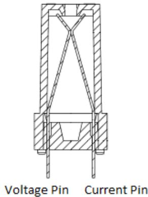
Fig. 4 Internal structure of a “kelvin contact” socket.
