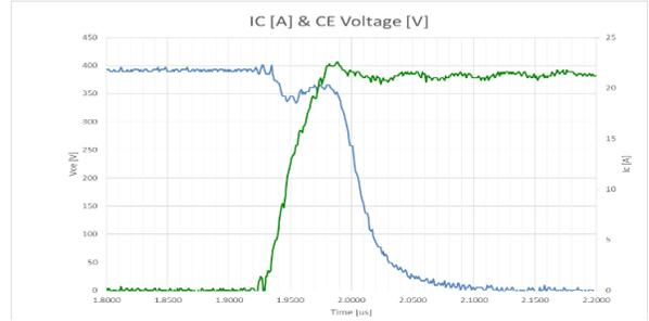
Fig. 7. Turn on waveforms collected with the developed measurement setup
