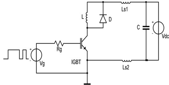
Fig. 5 Simplified circuit for switching test of the IGBT
