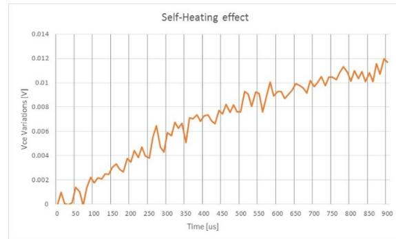
Fig. 3.  $V_{ce\_sat}$  variation versus time during the static test.
