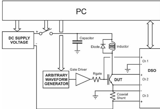
Fig. 2. Measurement system for dynamic characteristics.
