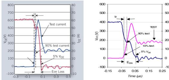
Fig. 6. Turn-on Loss Waveform for two different commercial IGBT.
