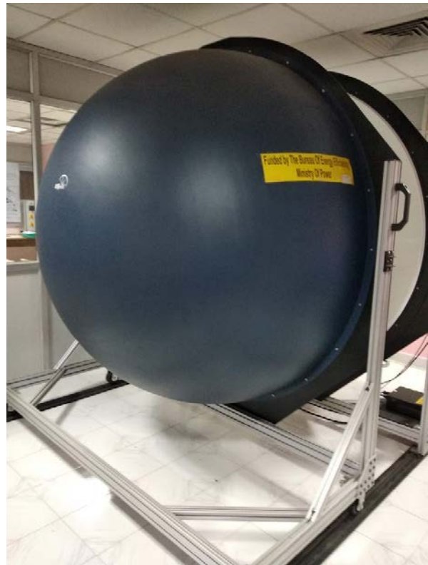
Figure 3: Labsphere 2m integrating sphere used for the measurement
