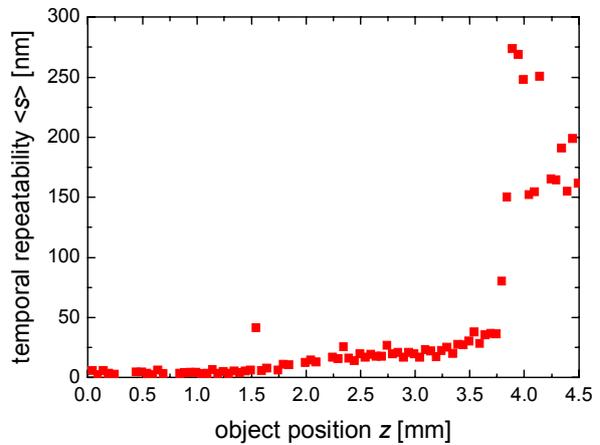
Fig. 8: Temporal repeatability of the OCT sensor as a function of the object position
