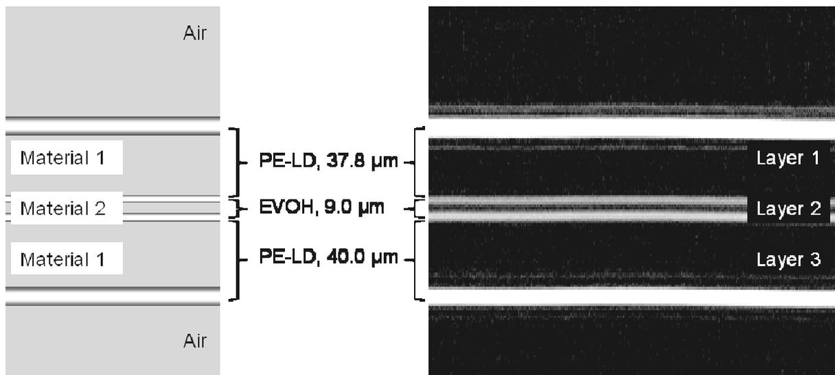
Fig. 9: Structure of a multilayer plastic film
