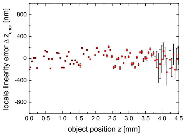
Fig. 7: Linearity error of the OCT sensor as a function of the object position
