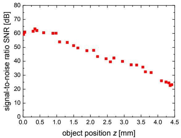
Fig. 6: Dynamic range of the OCT sensor as a function of the object position
