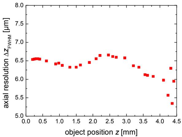
Fig. 5: Axial resolution of the OCT sensor as a function of the object position
