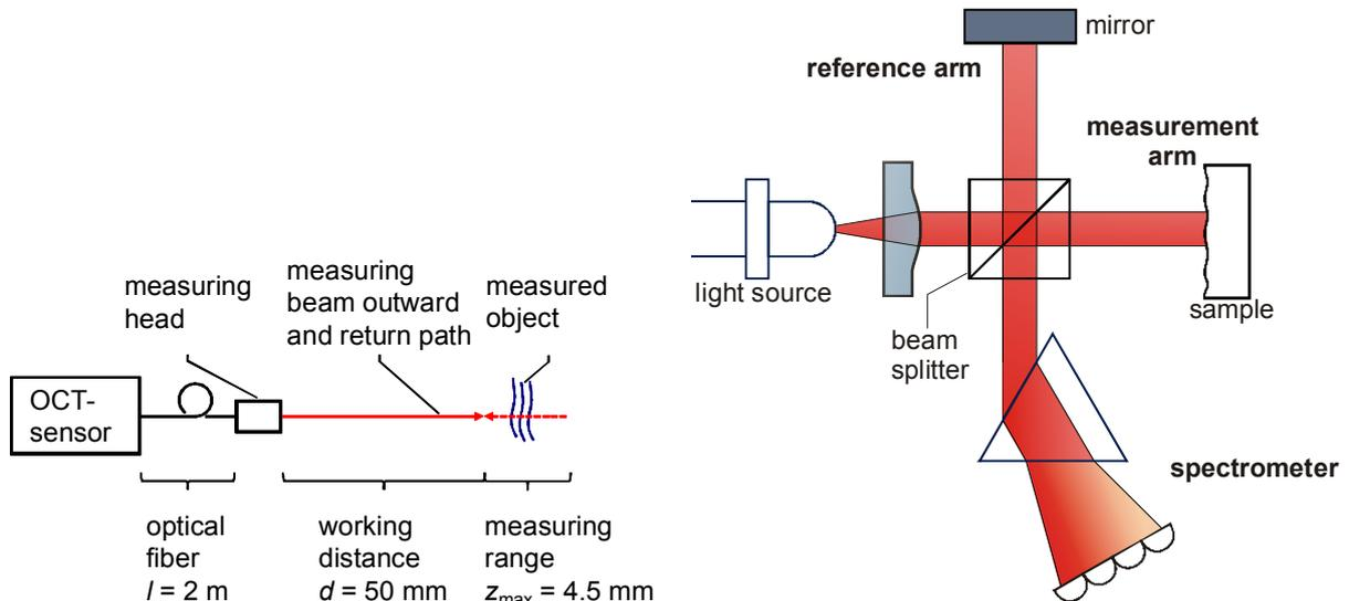
Fig. 3: Measurement set-up
