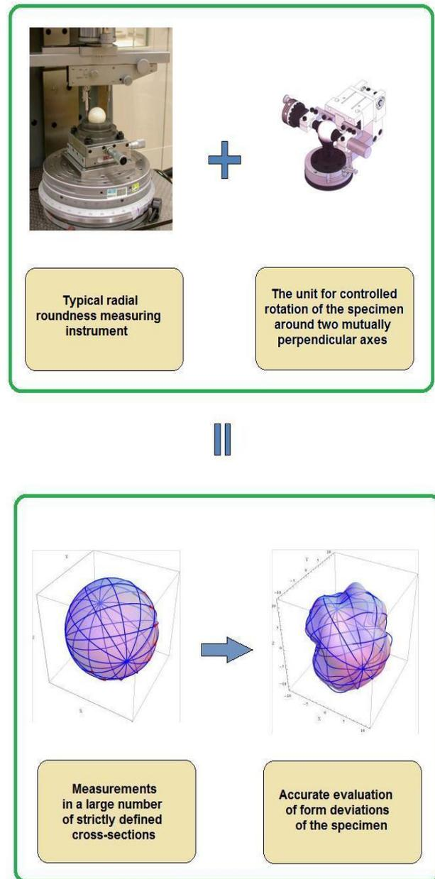
Fig. 1: The concept of the sphericity measurement by the radial method
