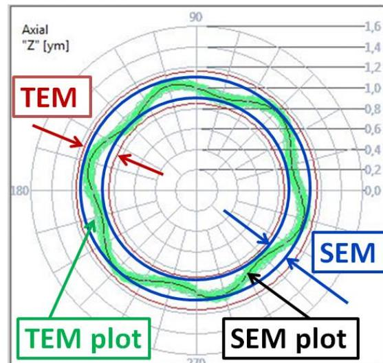
Fig. 1: Synchronous error motion AEM
