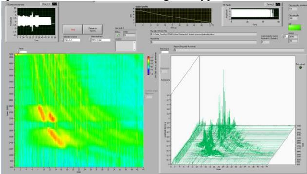
Fig. 7: Coast-down order analysis with intermittently self-excited vibrations - measured by displacement sensors
