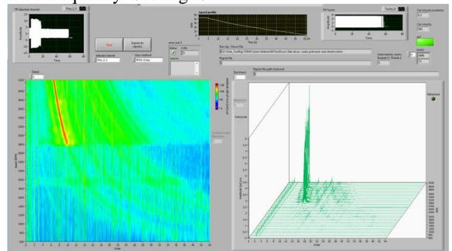
Fig. 6: Coast-down order analysis with continuously self-excited vibrations - measured by displacement sensors.
