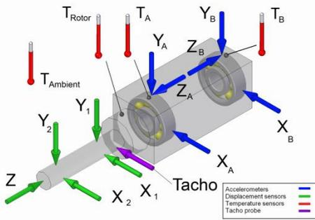
Fig. 4: Scheme of sensor application on the test rig
