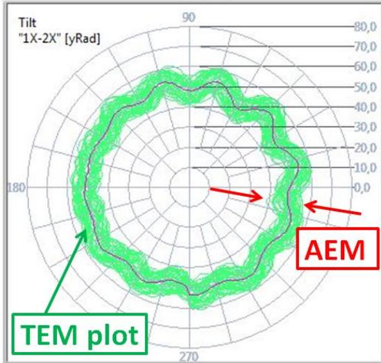
Fig. 1: Asynchronous error motion AEM
