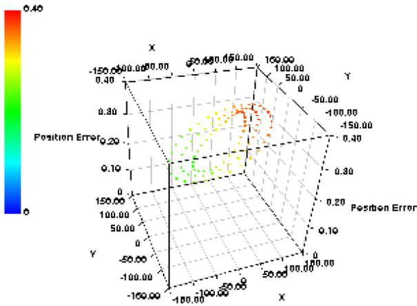
Fig.11: Position error at radius=50, 75, 100mm
