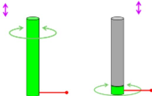
Fig.13: 2 rotating systems: left is stem rotation and right is unit rotation
