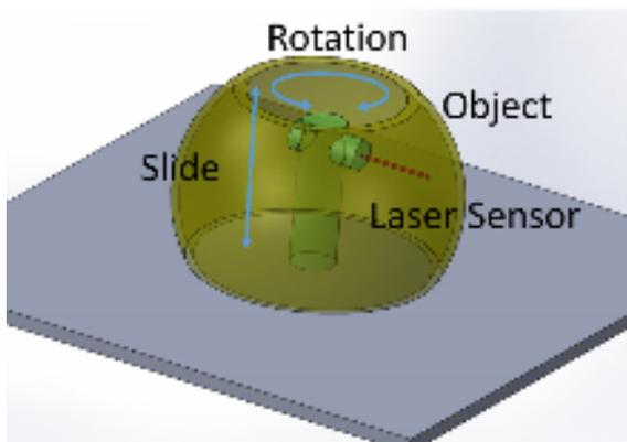
Fig. 1: Laser 3D measurement system
