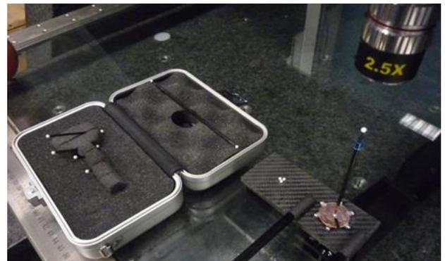
Fig. 7: Probing on a vertically placed miniature ball bar (right) according to the concept explained in Fig. 6
