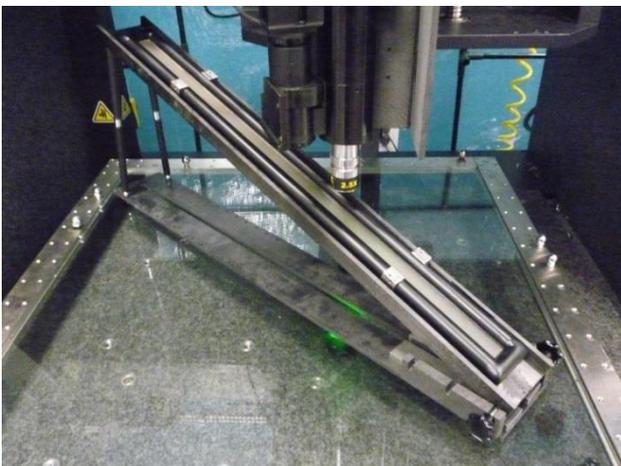
Fig. 4: Artefact on video CMM in space-diagonal placement; inclination device, holder full carbon fiber composite for thermal stability during measurement; support with “window” allows for backlight illumination; stability of inclinor achieved by using high modulus fibers, Continuous inclination angle variation due to magnetic telescopic rods of carbon fiber (left) and pivot axis (right)
