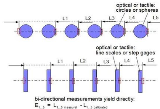
Fig. 1: Meaning of bi-directional length measurements
