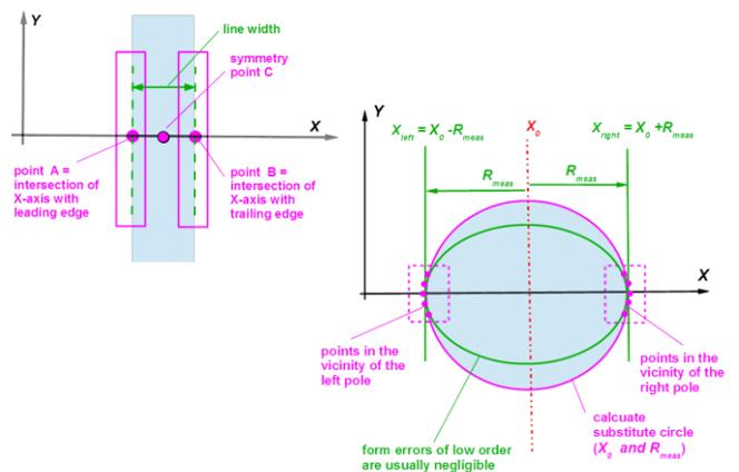
Fig. 2: Measuring lines and circles (centers and edges); the “trick” with dots is to measure around the poles and to add/subtract the measured radius to/from the center position
