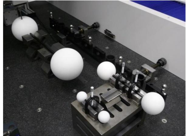
Fig. 8: Different dumbbell sizes, here dumbbells during tactile calibration; all balls with surfaces of fine-lapped paint
