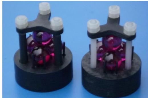
Fig. 12: Miniature tetrahedrons for tomography on stand; the springs of carbon fiber are so-designed that the balls are pressed together with equal forces, no glue needed, ruby
