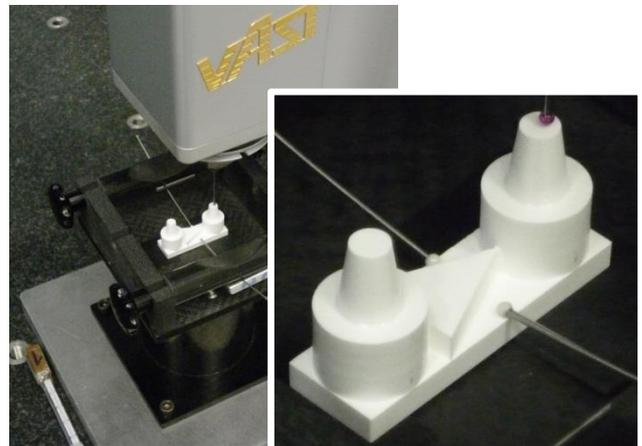
Fig. 10: Artifact for dental scanners during calibration (courtesy: [www.ISM3d.es](http://www.ISM3d.es))
