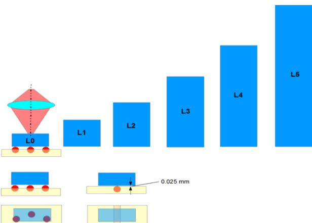
Fig. 5: Set up with gauge blocks, used in the past for verification of the Z-axis (optical axis); different weights of gauge blocks may cause elastic deformations in the supports
