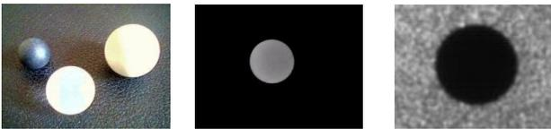
Fig. 12: Mat glass ball (left picture center) as a target for photogrammetry artefacts in comparison with ceramic ball (3rd ball from left), internally illuminated alumina ball (center picture), and black ball in front of reflex foil (right)
