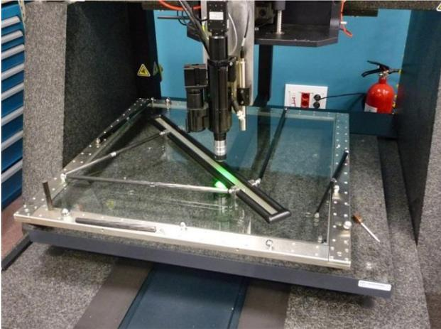
Fig. 3: Line scale of near zero thermal expansion on video CMM in XY-diagonal measurement line; case: “highly dynamic” table; stability is assured by magnetic rod fixtures in statically constrained arrangement
