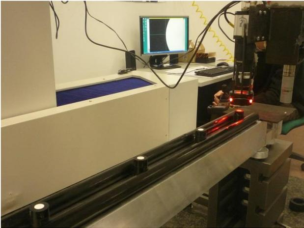
Fig. 11: Artifact for photogrammetry by the author, targets with plane surfaces and sharp circles during calibration (calibration set up: courtesy www.ism3d.es)
