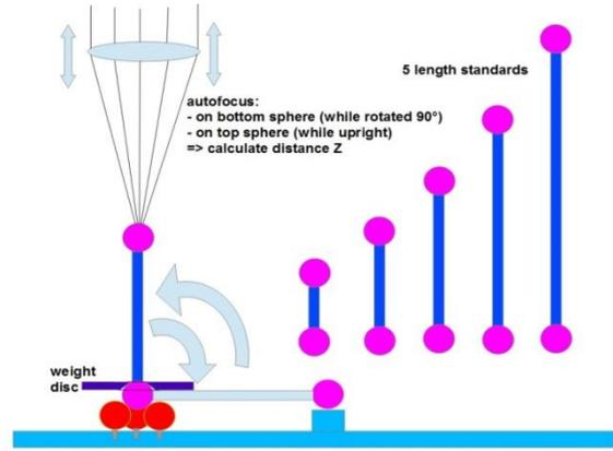
Fig. 6: Method for verification of the Z-axis; center on pole reflex, focus, 3D distance; black pigments deposited in the pores of the ceramic balls improves autofocussing
