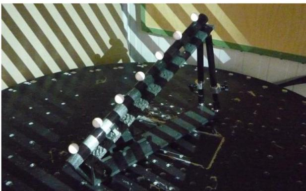
Fig. 9: Linear array ball beam with special low-volume scattering ceramics on fringe projection system
