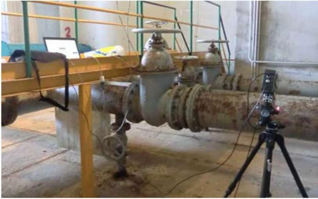
Figure 2 – Experimental set-up and pipe section of the water distribution network
