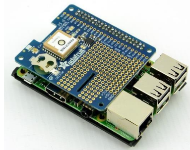
Fig. 4. Adafruit Ultimate GPS HAT plugged in Raspberry Pi
