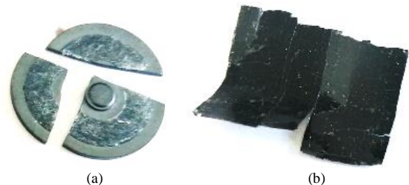
Fig. 2. Broken commercial ferrite shields (a) Solid shielded (b) Flexible shielded.
