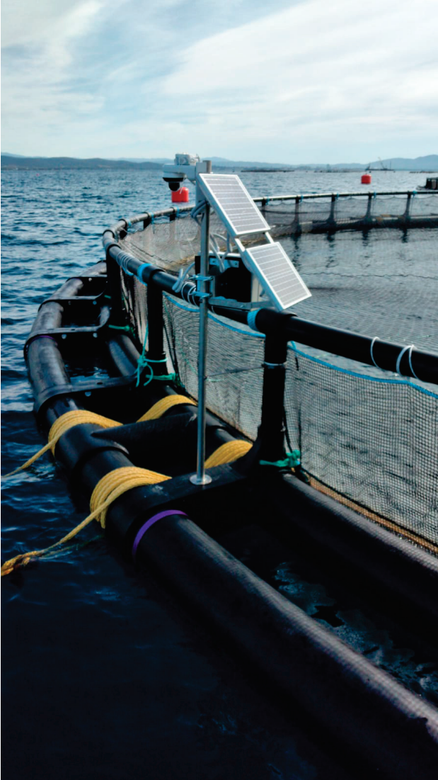
Fig. 3. Autonomous remote video monitoring system prototype offshore installed on a cage floating structure.
