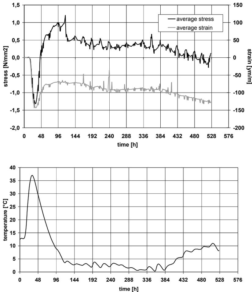
**Figure 6** Stress, strain and temperatur process into excavation rigid during the confirmation
