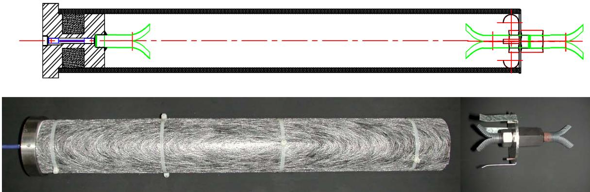
**Figure 1 Schematic representation of the sensor structure and photo**
