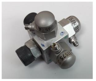
Figure 2: Cube tri-axial accelerometer showing the 10 mm<sup>3</sup> aluminium block, three ENDEVCO accelerometers and two M5 allen screw/nut counterweights
