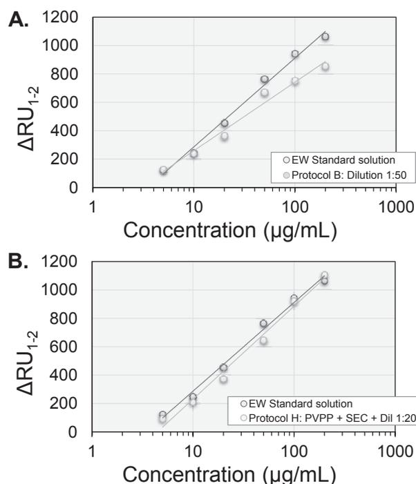
Fig. 2. Overlap of the calibration curves (matrix-matched vs standard), for two different purification protocols, resulting in rejection (panel A) and acceptance (panel B), respectively, of the null hypothesis  $H_0: b_{Matrix} - b_{Standard} = 0$ .
