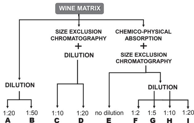
Fig. 1. Scheme of the sample preparation protocol designed and tested in order to reduce the matrix effect on the final analytical response.
