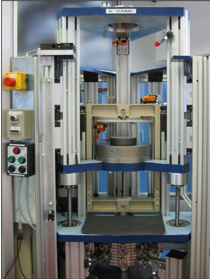
**Figure 1:** 2.5 kN force reference standard calibration machine
