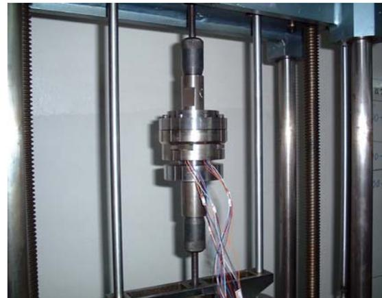
Fig. 12. Calibration setting for  $F_z$  component
