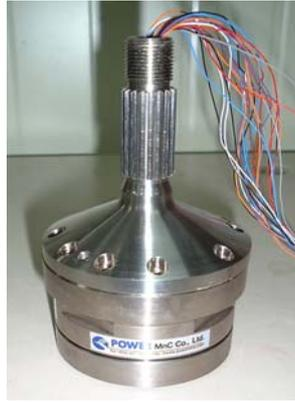
**Fig. 2. Sensing element and assembled load cell**
