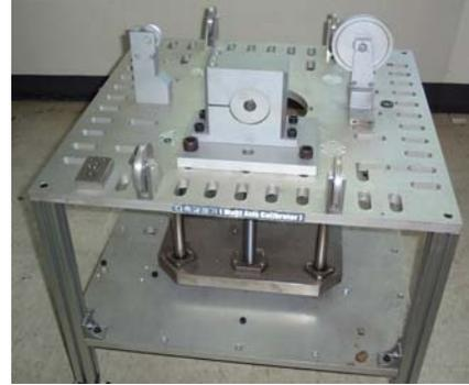
Fig. 11. Used multi-component force calibrator
