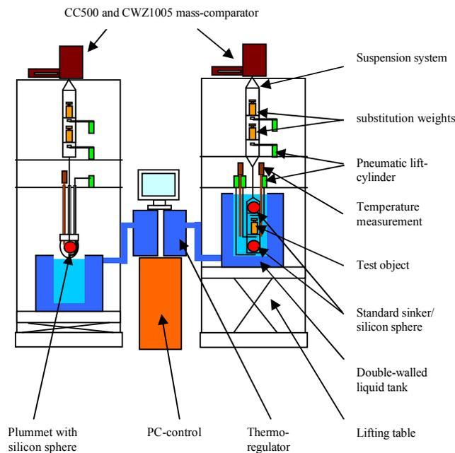
**Fig. 2:** Left: test station for measuring the density of liquids; right: test station for measuring the density of solids
