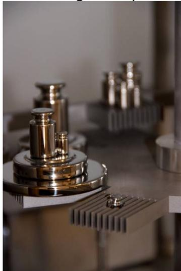
Fig. 13: weights from 1 g to 1 kg and also spheres can be carried directly
