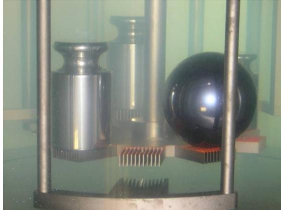
Fig. 17: comparison of a 1 kg, 500 g and 200 g test-weight with a national Volume standard (500 g Silicium sphere Nr. 2) of the BEV
