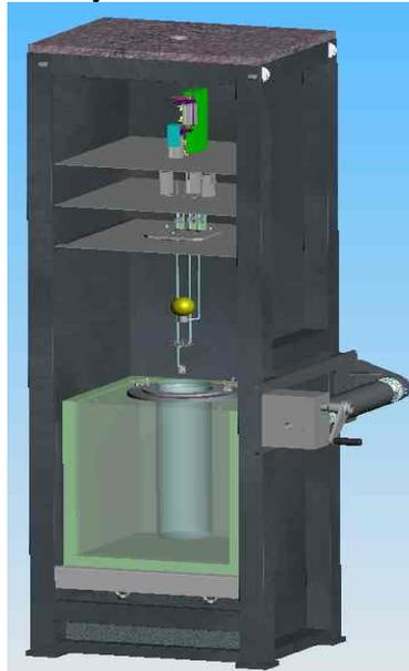
Fig. 4: Test station for measuring the density of solids in CAD
