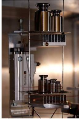
Fig. 6: Weight holder: lifting cylinder with mass comparator suspension system
