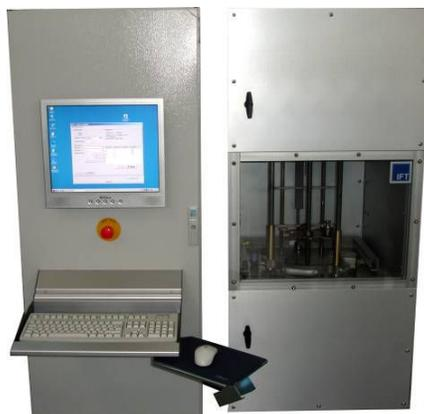
Fig. 9: Volume comparator VD1005: prototype at BEV
