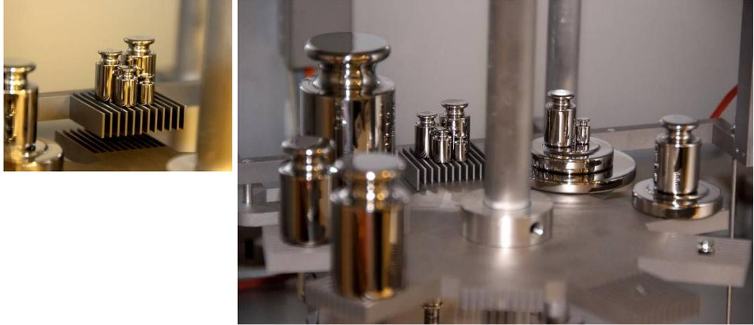
Fig. 13: Magazine for substitution weights: a couple of substitutions weights is lifted on the mass comparator suspension system
