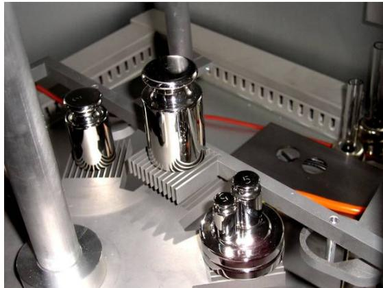
Fig. 14: a substitutions weights is lifted on the mass comparator suspension system; the positions system for the suspension system is opened.
