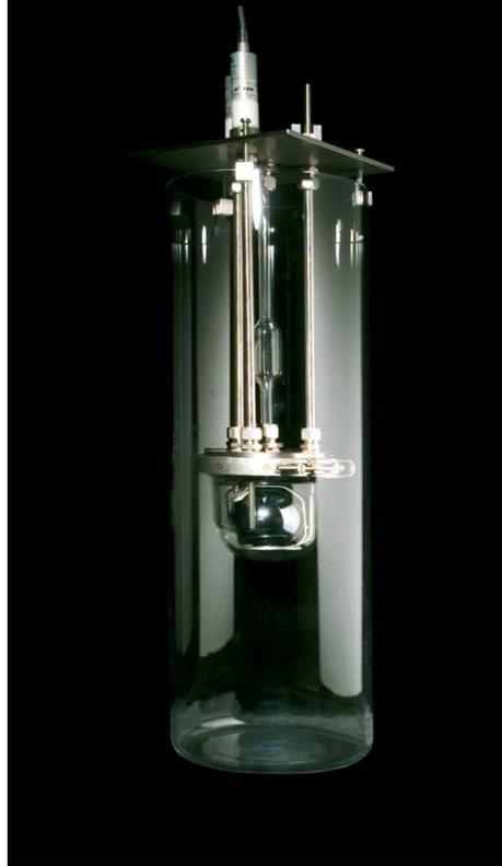
Fig. 5: determination of liquid density: measurement vessel with a bell-shaped chamber holding the silicon sphere before the thermostated bath is raised
