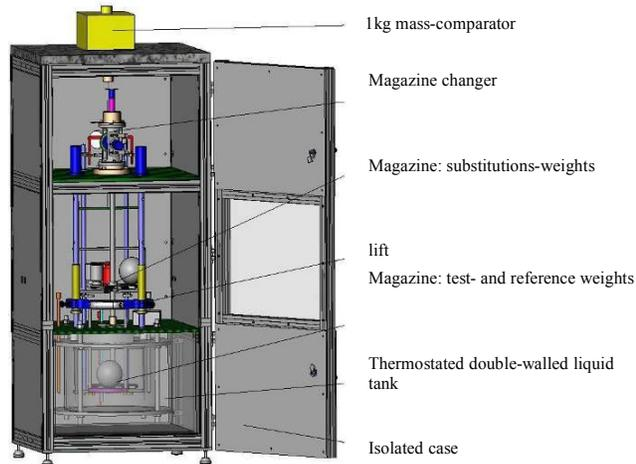
Fig. 10: CAD model of the volume comparator
