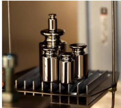
Fig. 7: Weight holder: a couple of substitutions weights is lifted from the mass comparator suspension system
