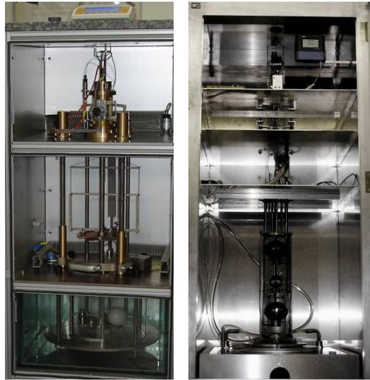
Fig. 2: The new volume-comparator (left) based on the new fundamental density aperture for solids (right) in the BEV; both are hydrostatic-below-weighing systems from 1g up to 1kg;
