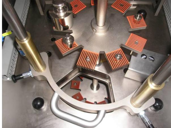
Fig. 12: Magazine for substitution weights, insertion mechanism, and view from above to the magazine in the weighing chamber
