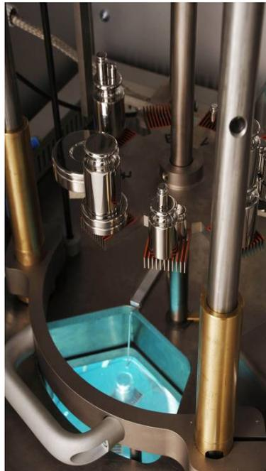
Fig. 16: calibration of a clients volume comparator in the BEV
