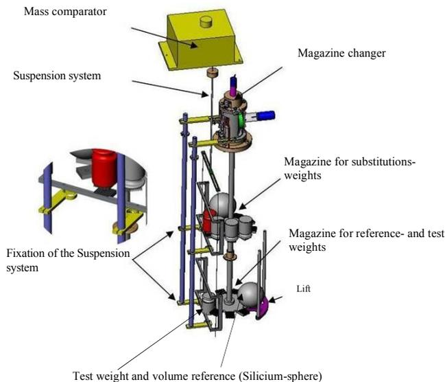
Fig. 11: CAD model of the transport unit
