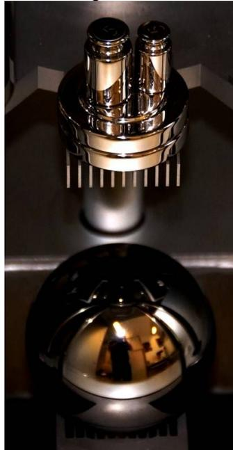
Fig. 1: The new volume-comparator: a Silicon volume standard and the corresponding substitutions weights
