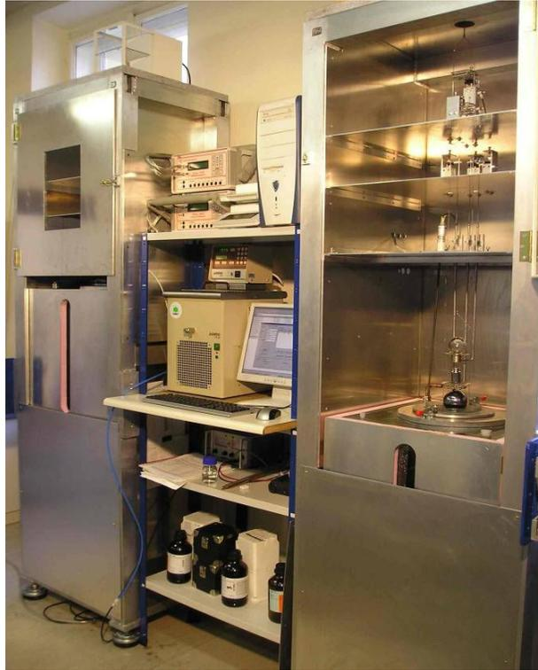
Fig. 8: System installed at BEV for the fundamental density determination
