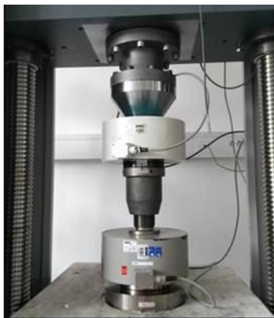
Fig. 1. Set-up of the machine for 600 kN range, compression, with control transducer on top, reference transducer mounted below it (in the middle) and transfer standard transducer at the bottom (all 600 kN).
