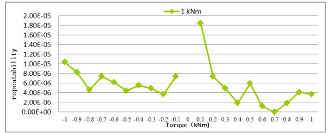
Fig.7 The results of repeatability test in 1kN·m segment
