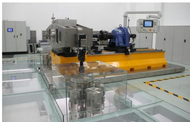
Fig.1 20 kN·m torque standard machine
