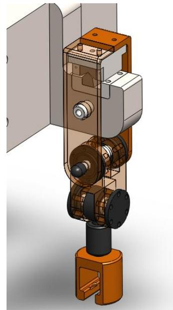
Fig.5 Weight suspension part
