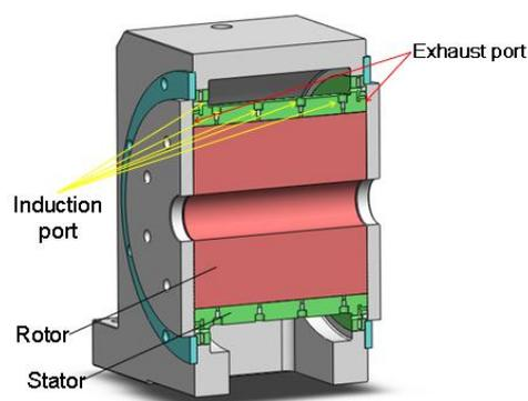
Fig.2 Structure of air bearing
