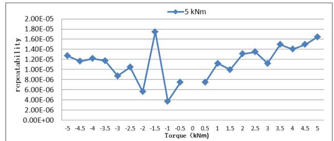
Fig.9 The results of repeatability test in 5kN·m segment
