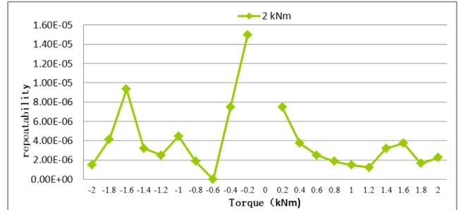
Fig.8 The results of repeatability test in 2kN·m segment
