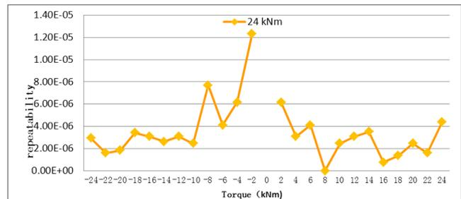
Fig.11 The results of repeatability test in 20kN·m segment
