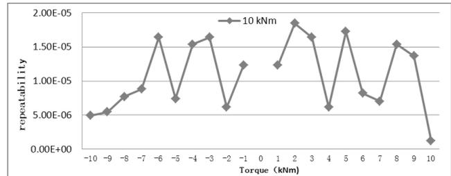
Fig.10 The results of repeatability test in 10kN·m segment
