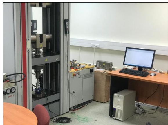
Figure 3: Zwick material testing machine and calibration systems
