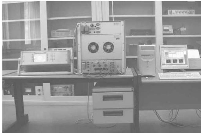
Fig 4 Picture of the system for the comparison of three-phase wattmeters
