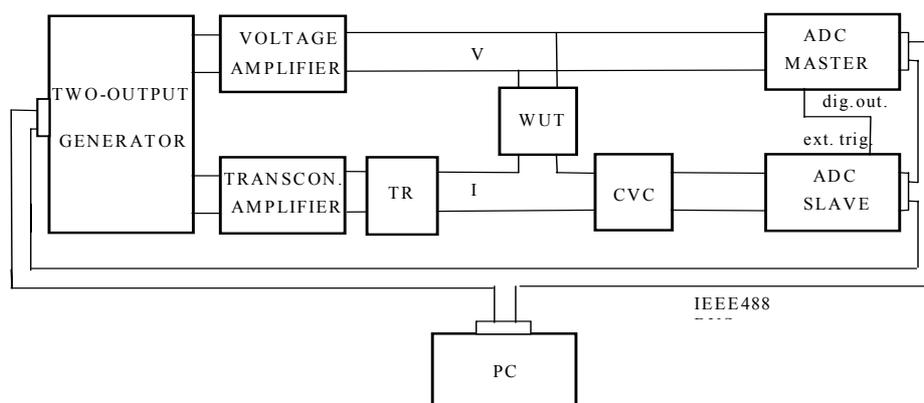
Fig. 1 Basic scheme of the system for the primary measurement of electrical power connected for the calibration of a wattmeter under test (WUT). TR is the transformer for selecting the output current, CVC is the current to voltage converter.
