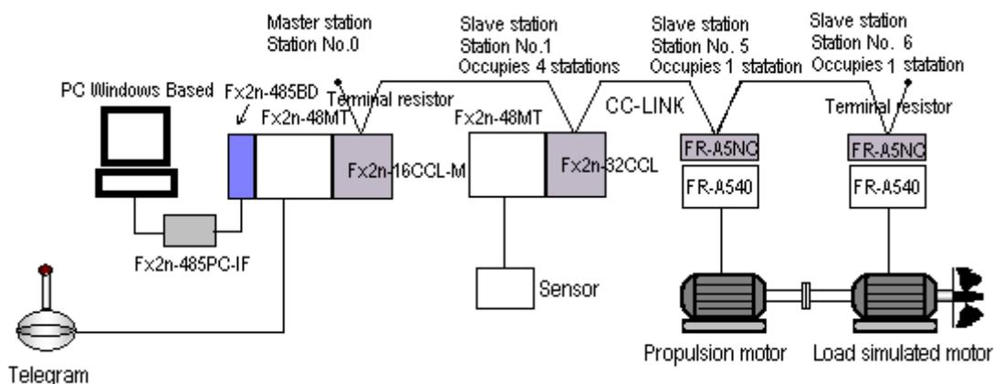
Fig.1. Measurement Platform structure based on CC-Link
