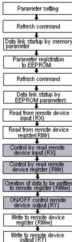
Fig.2. The basic programming procedure flowchart for parameter setting
