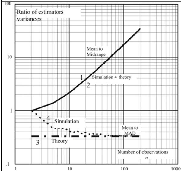
Fig. 5a Efficiency of rectangular distribution: estimators as functions of number  $n$  of observations (Monte Carlo simulation by  $200 \times 2^{20}$  random numbers [5]). Ratio of mean value and midrange variances  $s^2(\bar{x})/s^2_{v/2}$ : (1)  $\approx$ (2) - theoretical function  $(n+1)(n+2)/6n$  from [9] and curve from simulation. Ratio of mean value and of median MAD variances  $s^2(\bar{x})/s^2_{MAD}$ : (3) - theoretical function =  $1/3$ , (4) - curve from simulation.
