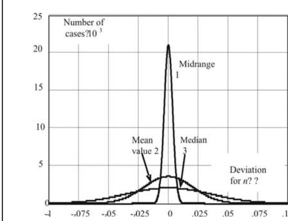
Fig. 5b Histograms of estimators of the rectangular distribution (-0.5...+0.5) simulated by  $200 \times 2^{20}$  random numbers [5]: 1 - midrange; 2 - mean value; 3 - median.
