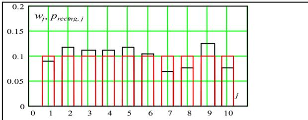
Fig.4. Histogram of the example 2 observations: black -  $w_j$  of sampled observations; red -  $p_{rectng,i}$  of rectangular distribution. The smallest and highest observations: 2.469...1.105 Number of histogram classes:  $m=10$  of 0.864 width
