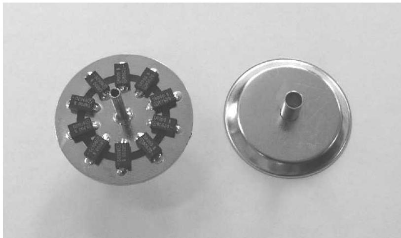
Fig. 4 Internal disk and cover of the shunts for currents from 100 mA to 2 A.
