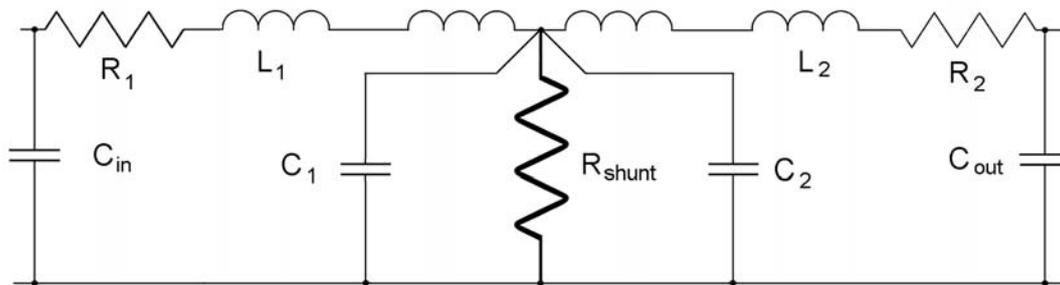
Fig. 1 Simplified circuit of the shunts
