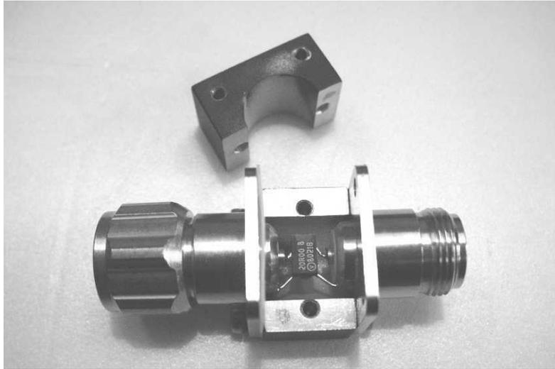
Fig. 2 Photograph of a shunt for 50 mA.
