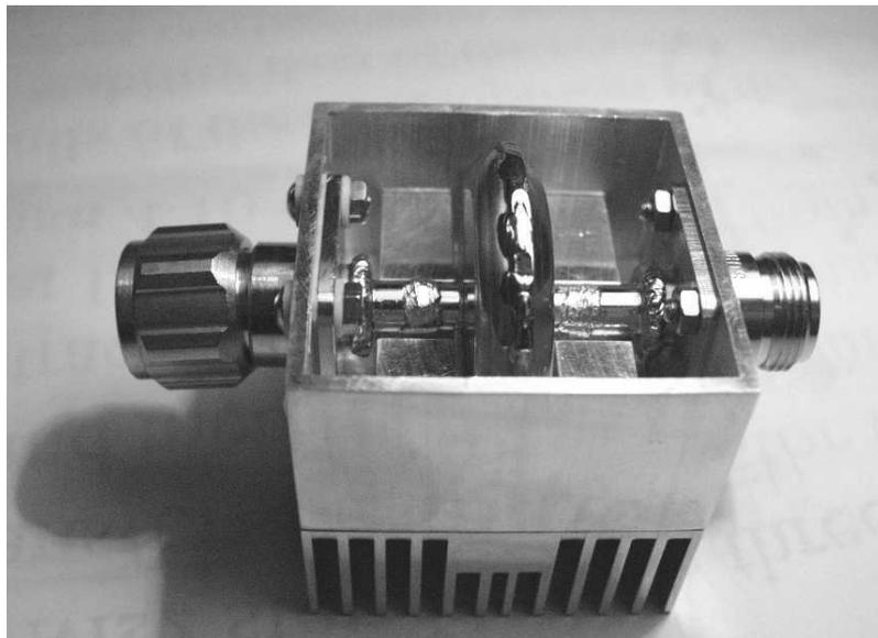
Fig. 5 Photograph of a shunt for 2 A.
