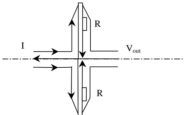
Fig. 3 Basic scheme of the shunt with the current path.
