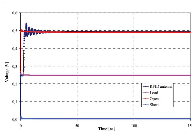
Figure 5. Zoom-in of the TDR waveforms for the ALR-8610 AC and for the calibration measurements
