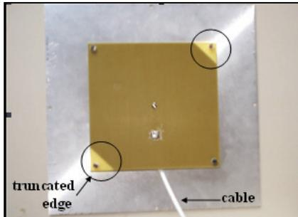
Figure 1. Picture of the RFID antenna under test
