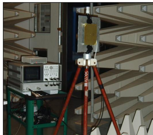
Figure 4. Set-up for the measurement carried out in the anechoic chamber
