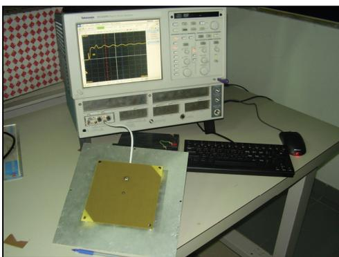
Figure 3. Set-up for the TDR-based antenna measurements
