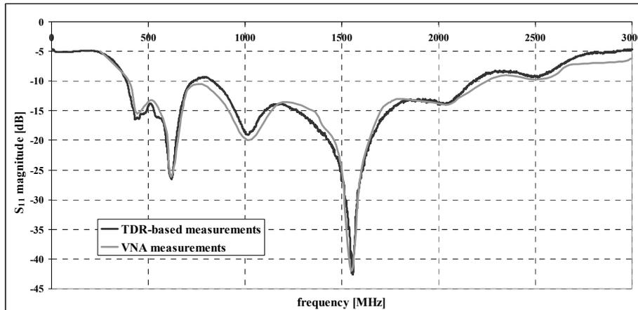
Figure 7. Comparison between the  $S_{11}$  (magnitude) for the biconical antenna under test
