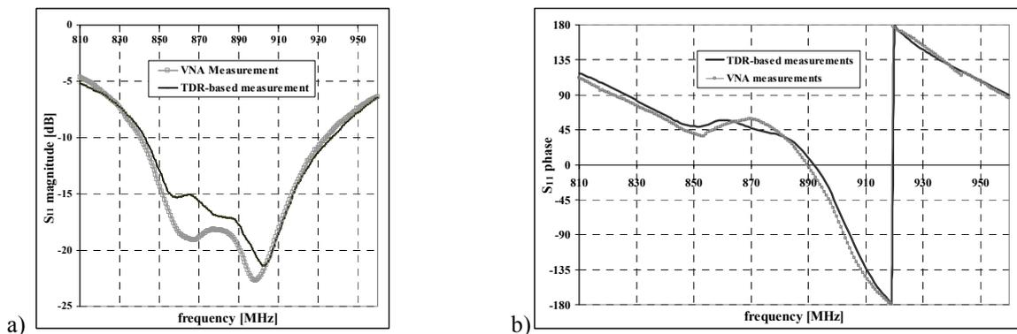
Figure 6. Comparison between the  $S_{11}$  obtained through FD transformation of TDR data (black curve) and through VNA measurements in anechoic chamber (grey curve) a) in magnitude, b) phase
