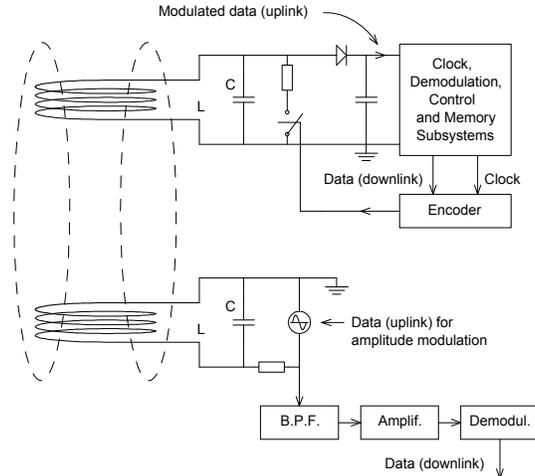
Figure 2. Inductive coupling with load modulation working principle.
