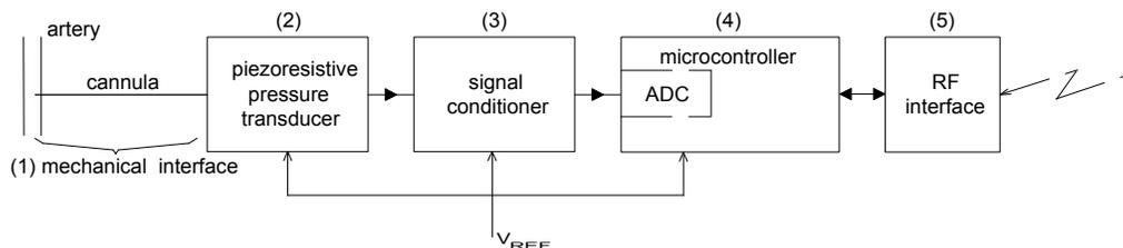
Figure 4. Implant's conceptual model.
