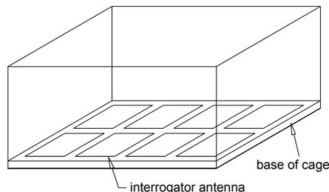
Figure 5. Several coupling inductors in the cage of laboratory animal.
