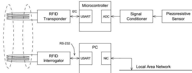
Figure 3. The arterial pressure measurement system.
