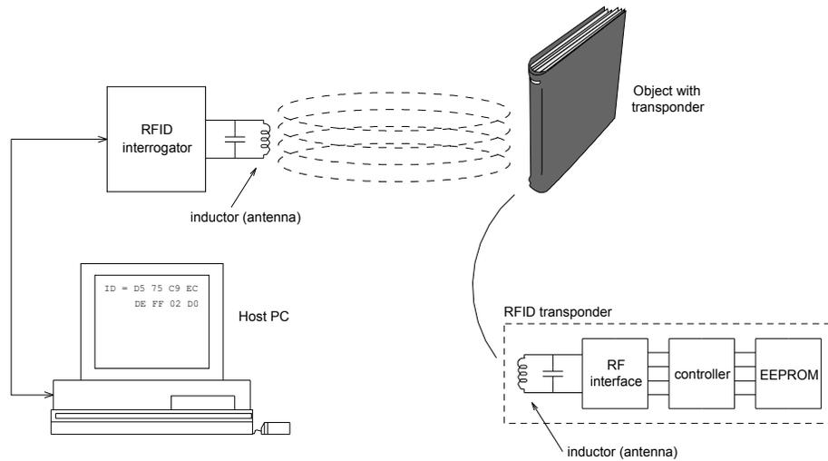
Figure 1. Typical RFID system.
