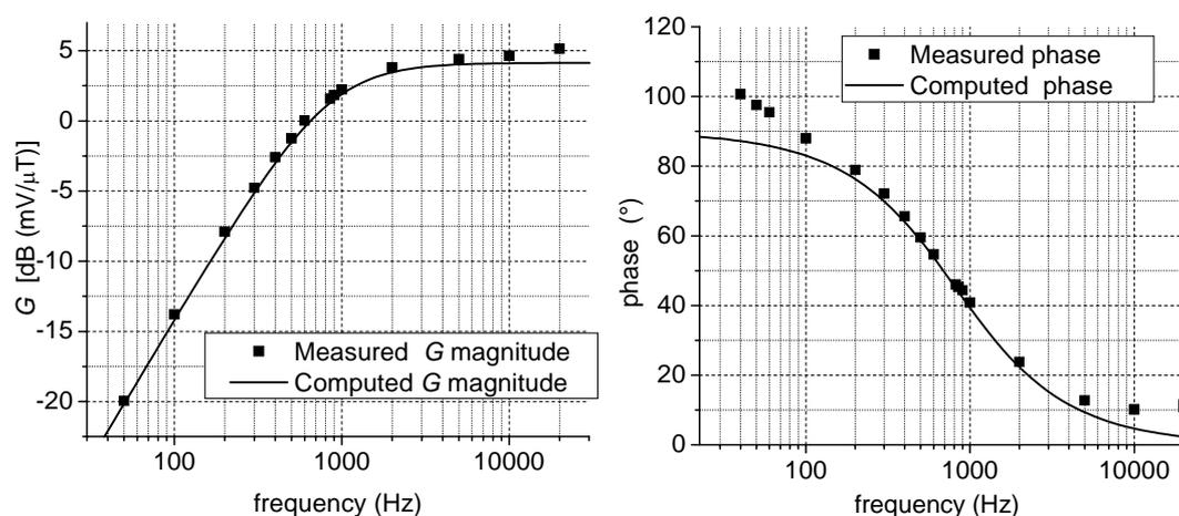
Fig. 8 – Comparison between the measured and computed magnitude and phase of the gain of the system reported in Fig. 7.
