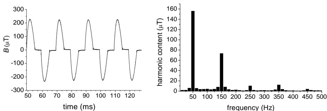
Fig. 1 – Magnetic flux density measured during spot resistance welding and related harmonic content.
