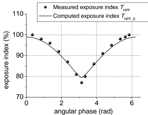
Fig. 5 – Influence of the third harmonic phase on the exposure index evaluated by the high pass filter approach.
