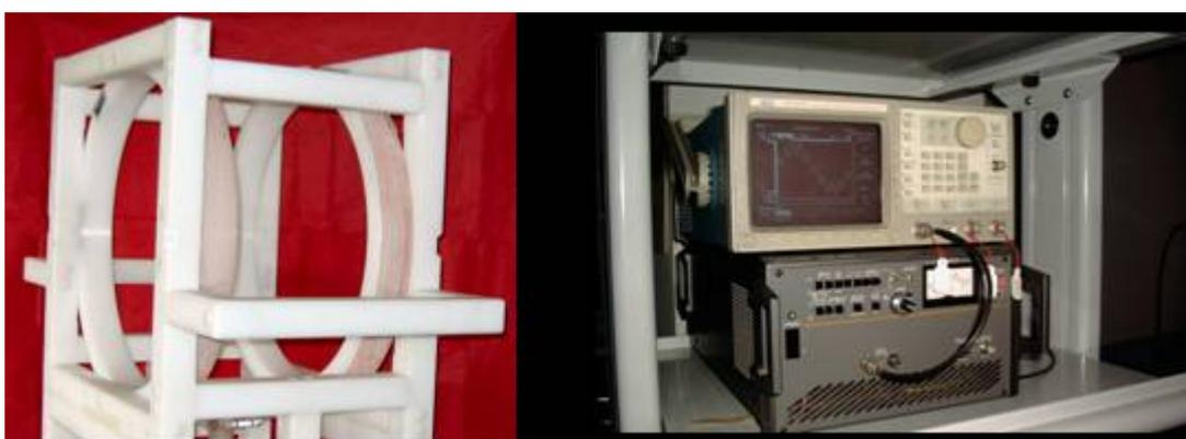
Fig. 3 – INRIM set up for the generation of sinusoidal and distorted reference magnetic fields up to 100 kHz.
