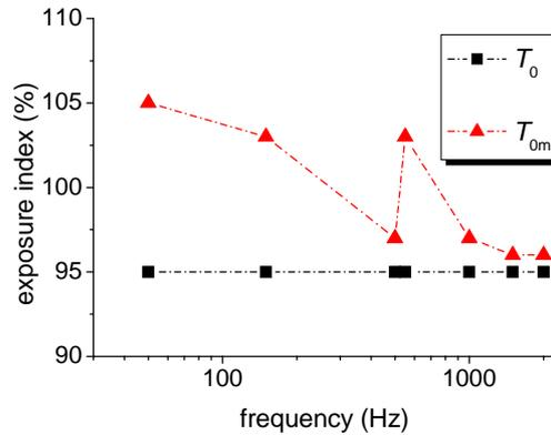
Fig. 6 - Comparison between the exposure index associated with the generated field ( $T_0$ ) and that measured ( $T_{0m}$ ) by a meter which performs the analysis in the frequency domain
