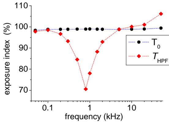
Fig. 4 – Exposure index in presence of sinusoidal fields evaluated by the same meter through conservative ( $T_0$ ) and high pass filter weighting approach ( $T_{HPFF}$ ).
