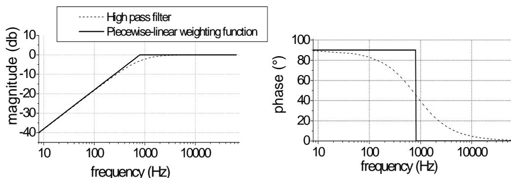
Fig. 2 – Piecewise linear and first order high pass filter magnitude and phase weighting functions (reference frequency  $f_{ref} = 50$  kHz).
