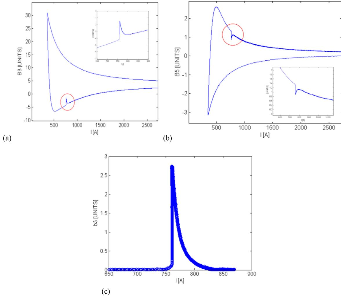
Figure 5. b3 (a) and b5 (b) decay and snapback; b3 snapback (c) after the data processing.
