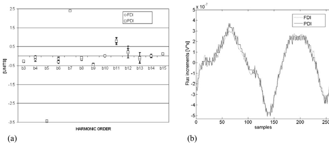
Figure 3. Average magnetic flux harmonics with 3- $\sigma$  bar (a), and compensated flux increments (b) at warm conditions, measured by the new FDI-based and the old PDI-based platforms.
