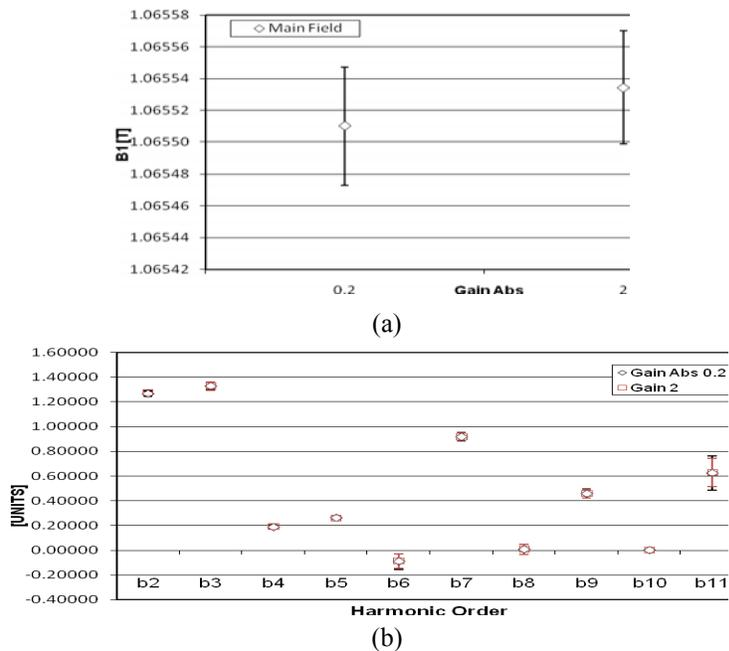
Figure 4.  $B_1$  mean (a) and high-order harmonics mean (b) with  $3\text{-}\sigma$  bar for two different FDI gains.
