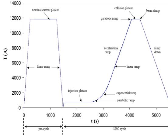
Figure 2 . LHC current cycle.
