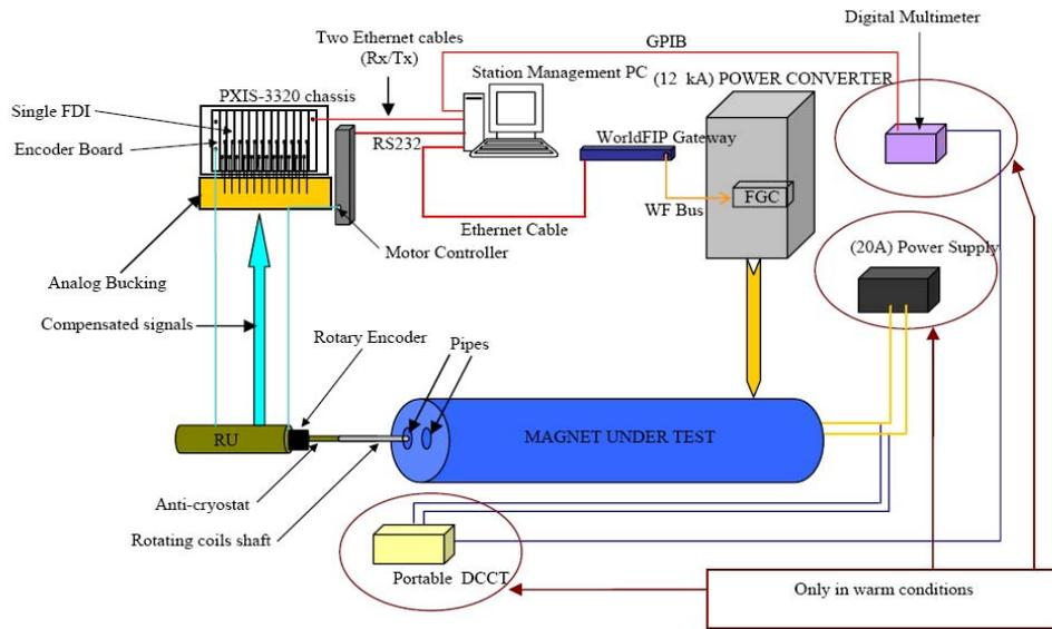
Figure 1. Test station for the platform on-field characterization.
