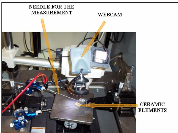
Figure 1: The implemented measurement system for the electric resistance measure
