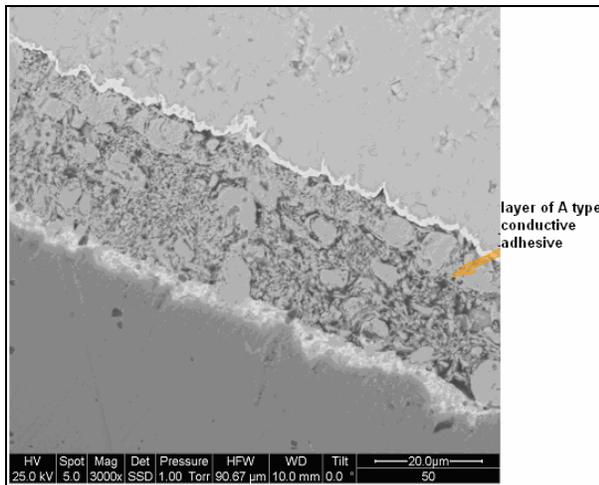
Figure 6: polymerized (@80°C) A type conductive
