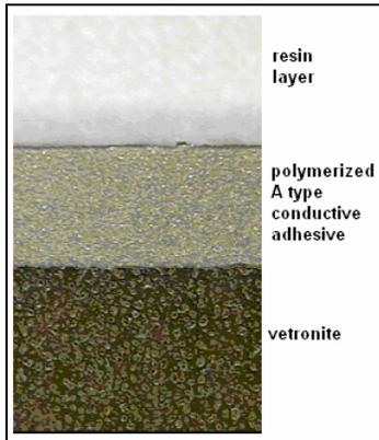
Figure 4: layer of polymerized (@80°C) A type conductive adhesive of 50  $\mu\text{m}$
