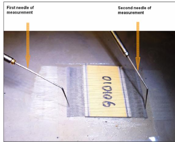
Figure 2: Detail of the system for the electric resistance measure
