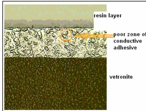
Figure 5: layer of polymerized (@80°C) B type conductive adhesive of 50  $\mu\text{m}$ , localization of poor zone.
