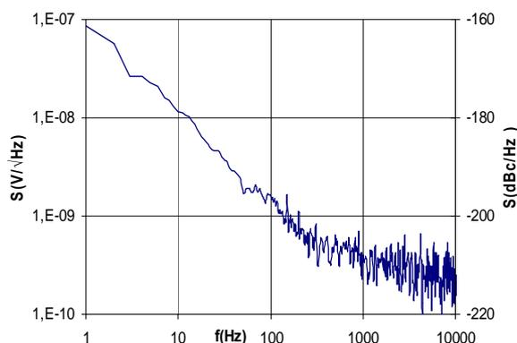
Figure 7. Frequency spectrum on the output of the power supply at operation from internal accumulator.
