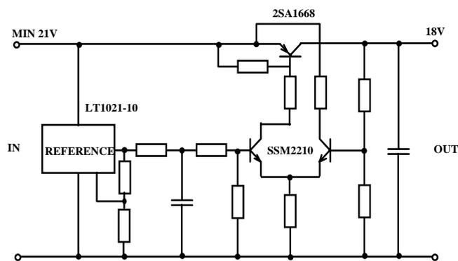
Figure 4. Discrete transistor DC voltage regulator
