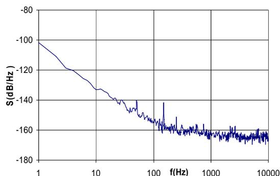
Figure 3. The output voltage noise spectral density of the HP 3631a power supply standardized to output voltage.
