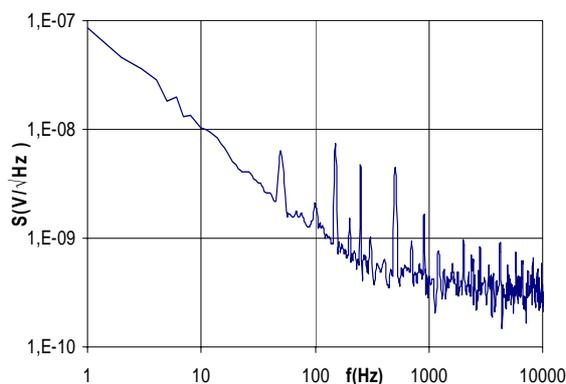
Figure 8. Frequency spectrum on the output of the power supply at operation of the power net.
