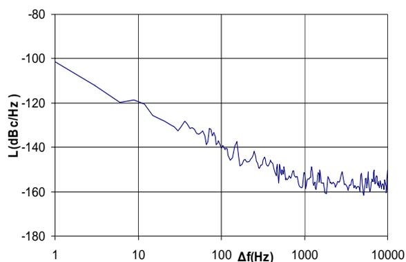
Figure 1. Phase noise power spectrum of the LN oscillator powered from the power supply HP 3631a
