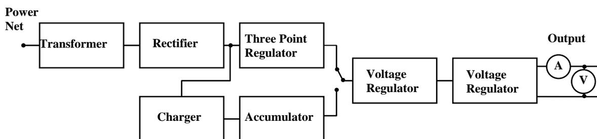
Fig.5 The block diagram of the power supply
