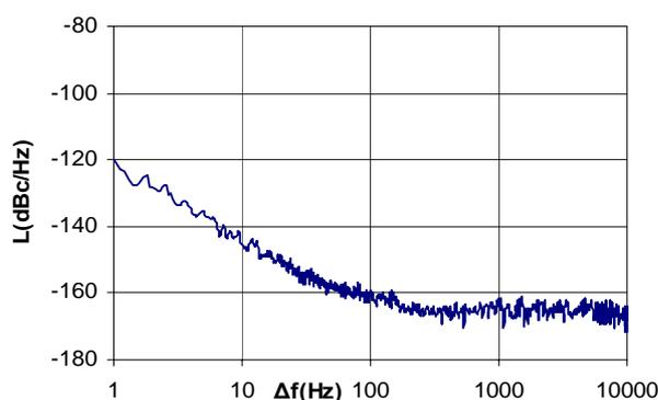
Figure 2. Phase noise power spectrum of the LN oscillator powered from the accumulator
