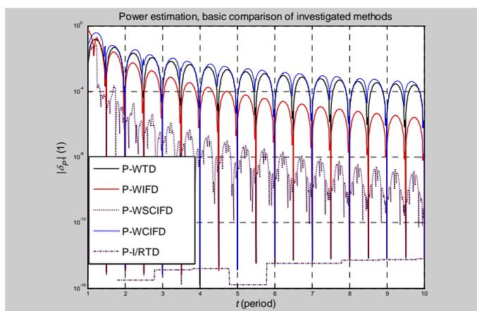
Fig. 1. Dependence of relative bias of active power estimation by the inspected methods on sampling time expressed in input signal periods
