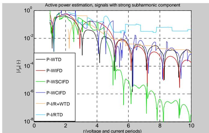
Fig. 2. Dependence of relative bias of active power estimation by inspected methods on sampling time expressed in input signal periods
