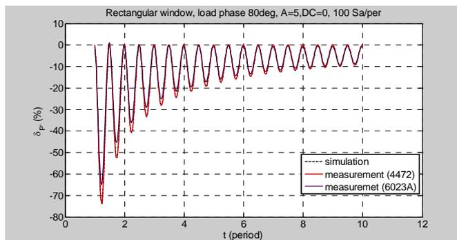
Fig. 3. Comparison of relative bias of active power estimation gained by simulation and by measurement.
