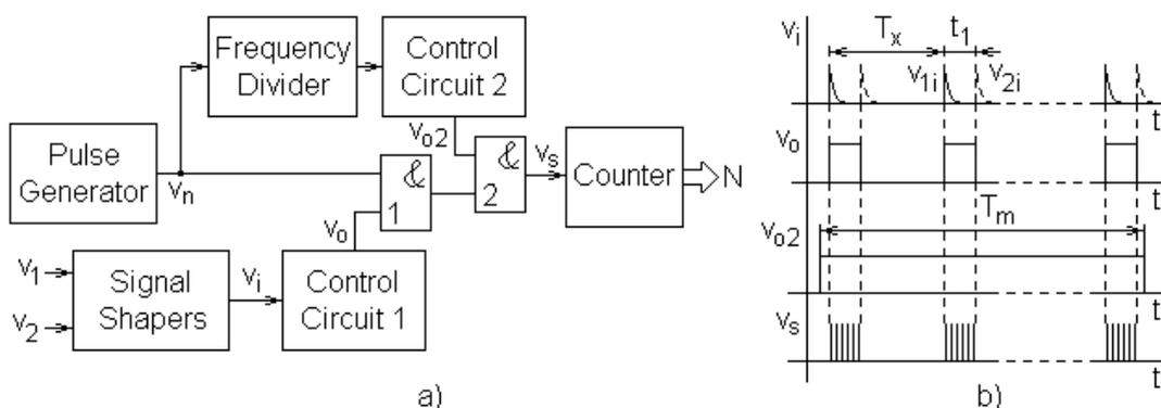
Figure 1. Measurement of the average phase angle value: a) block diagram, b) time diagrams
