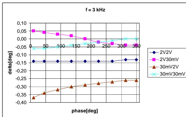
Figure 6. Phase measurement error, f = 3 kHz
