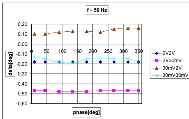
Figure 4. Phase measurement error, f = 50 Hz
