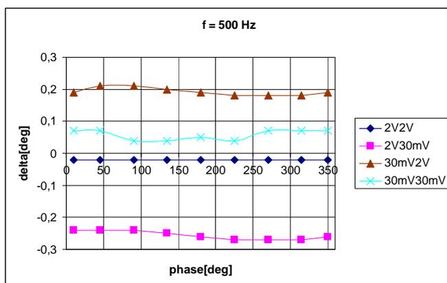
Figure 5. Phase measurement error, f = 500 Hz
