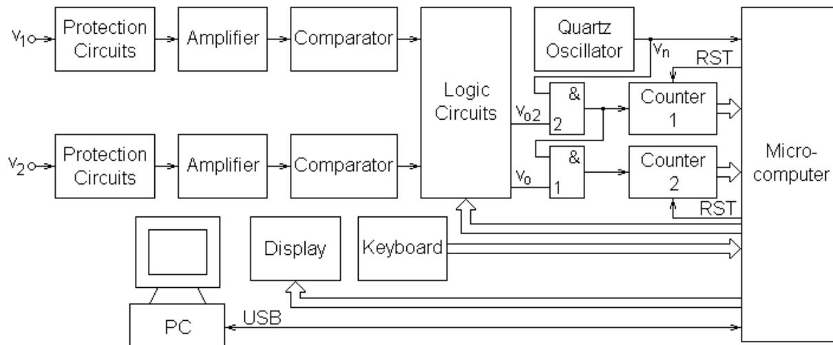
Figure 2. Block diagram of the designed low-frequency digital phase meter
