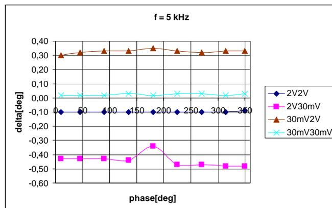
Figure 7. Phase measurement error,  $f = 5$  kHz
