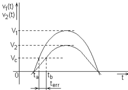
Figure 3. Time error caused by different signal levels
