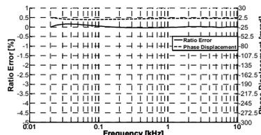
Figure 3. Ratio error and phase displacement of compensated current transformer.
