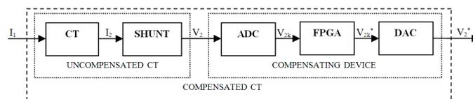
Figure 2. Block scheme of the compensated current transformer
