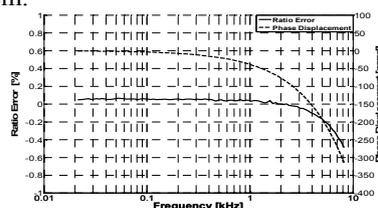
Figure 1. Ratio error and phase displacement of the realized transducer.
