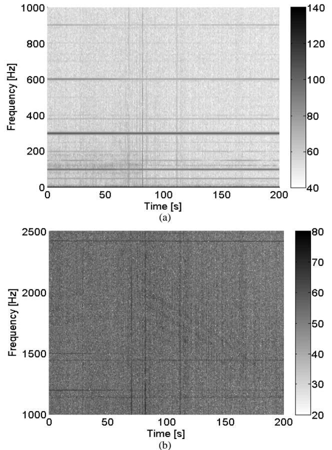
Figure 4. Spectrogram: (a) low frequency steady harmonics; (b) higher frequency range including time-varying harmonics
