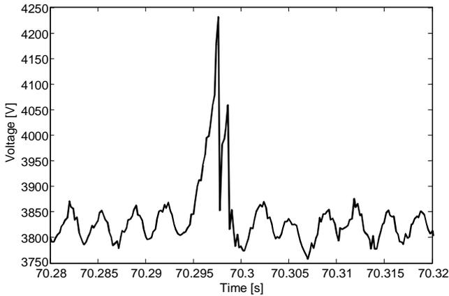
Figure 9. Waveform of the  $V_p$  transient analyzed in Fig. 8
