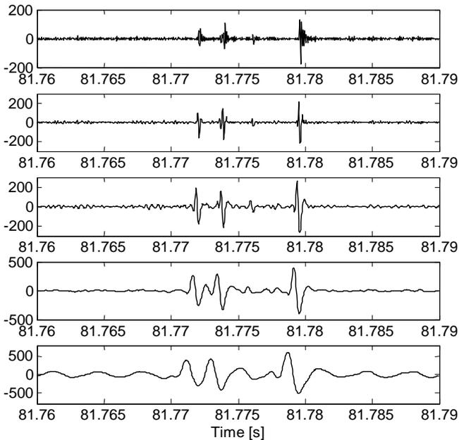
Figure 10.  $V_p$  transient of Fig. 6:  $db3$ , 5 levels wavelet
