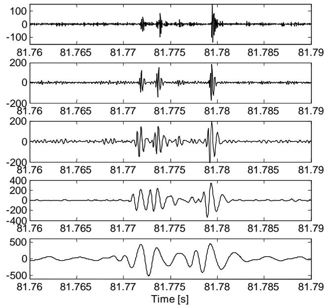
Figure 12.  $V_p$  transient of Fig. 6:  $db8$ , 5 levels wavelet (similar to  $db10$  and various high order *sym* wavelets)
