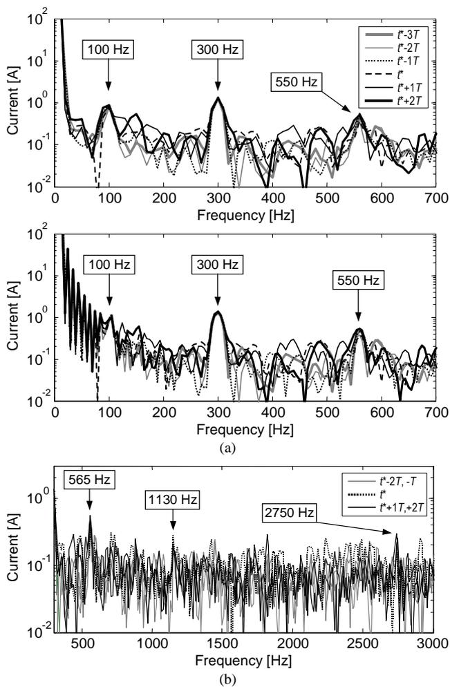
Figure 3. Analysis of transient behavior at  $t^*=5.8$  s (a) low frequency, with base and enhanced frequency resolution; (b) high frequency
