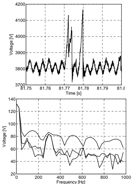
Figure 6. Spectrogram: transient waveform and Fourier spectra before, at and after the transient (20 ms time step)
