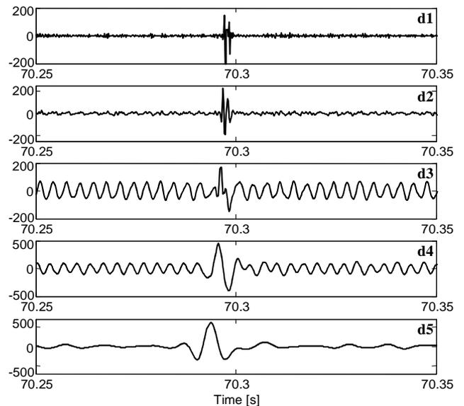
Figure 8. Example of  $V_p$  transient analyzed with *db3*, 5 levels wavelet
