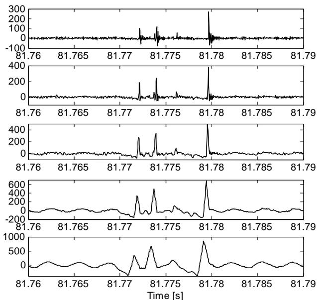
Figure 13.  $V_p$  transient of Fig. 6: *db1*, 5 levels wavelet (identical results for *sym1* and *haar* wavelets)
