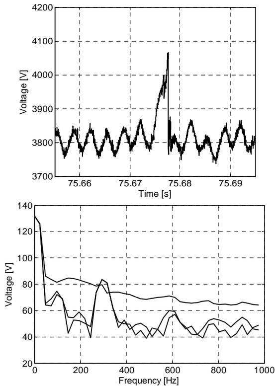
Figure 5. Spectrogram: transient waveform and Fourier spectra before, at and after the transient (20 ms time step)
