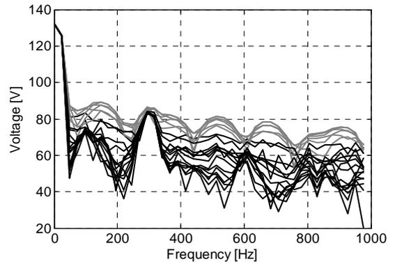
Figure 7. Spectrogram (refinement of the analysis of Fig. 6): spectra before (dashed black), partially including (solid black), centered at (solid gray) and after (dotted black) the transient (4 ms time step)
