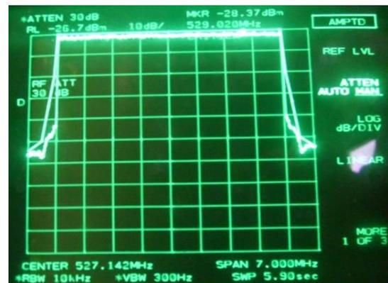
**Fig. 10a critical mask measurement**
