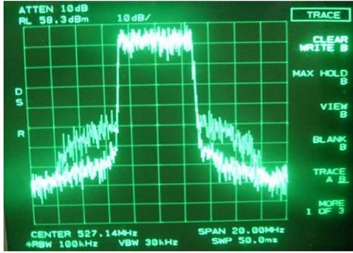
Fig. 3 spectral growth caused by the input mixer level.
