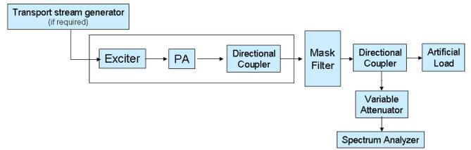
Fig. 8 ISDB-T characterization block diagram between the  $\pm 3\text{MHz}$  from the center frequency
