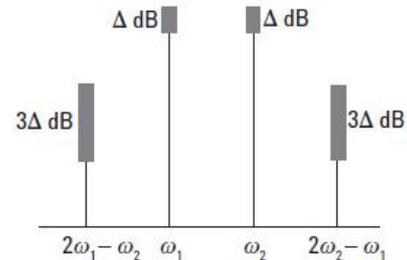
Fig. 2 two tone intermodulation
