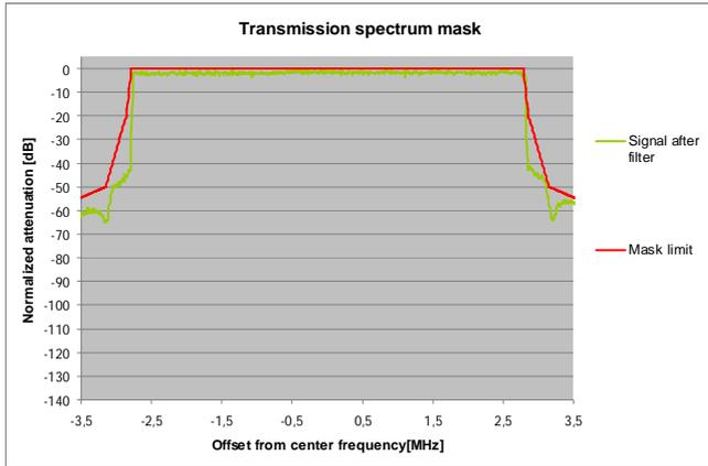
Fig. 10b critical mask measurement between ±3.5MHz from the channel center frequency
