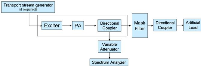
Fig. 6 ISDB-T characterization block diagram.
