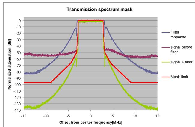
Fig. 12 Transmission spectrum mask measurement results
