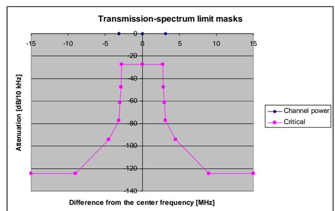
Fig.1 ISDB-T critical mask
