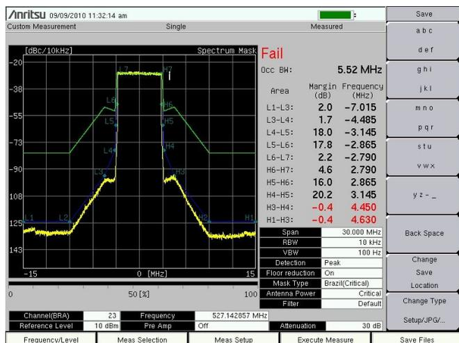
**Fig. 13 Transmission spectrum mask measurement results using default filter**
