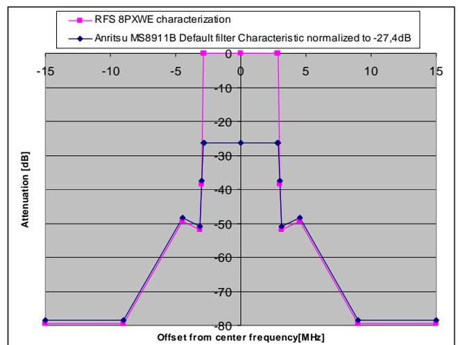
Fig. 9 Anritsu 8911B default filter comparison.
