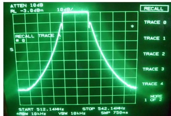
Fig. 5b filter characterization trace.
