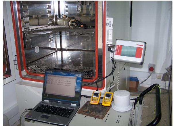
Fig. 1. Calibration system for temperature
