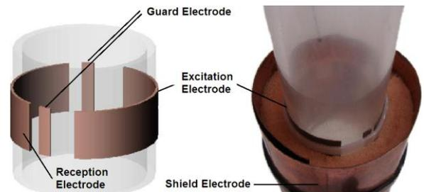
Fig. 1. Capacitive Probe
