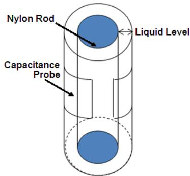
Fig. 9. Annular flow calibration scheme.
