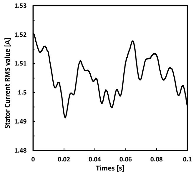
Fig. 8 RMS value of the stator current a motor without rotor eccentricity.
