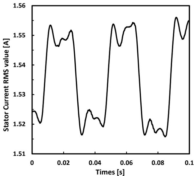
Fig. 9 RMS value of the stator current of a motor with rotor eccentricity.
