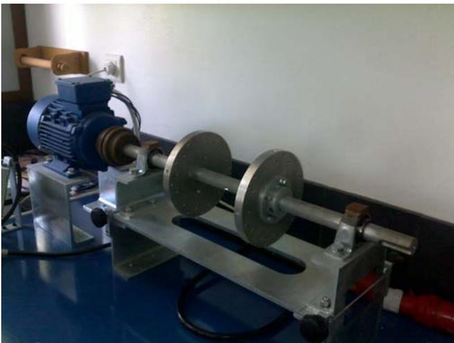
Fig. 2. Induction motor and adjustable shaft used to test rotor eccentricity faults.
