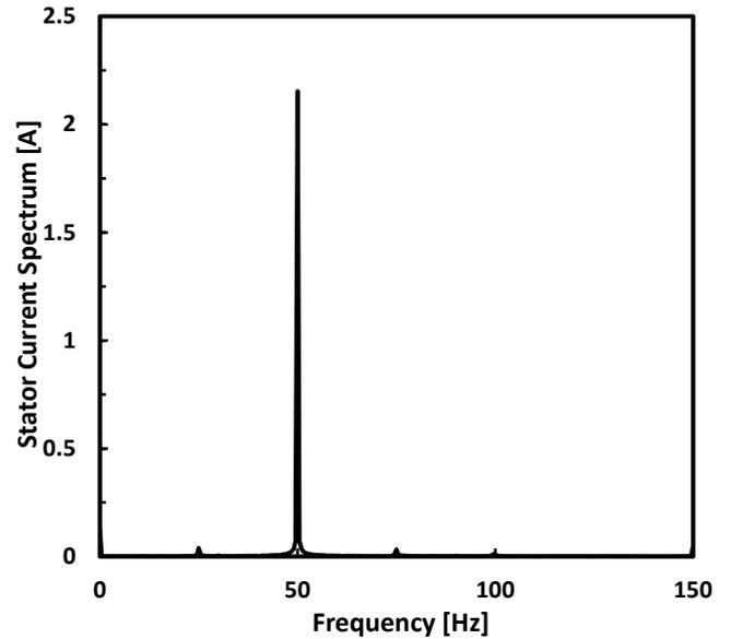
Fig. 7 Amplitude spectrum of the acquired stator current of the machine with rotor eccentricity.
