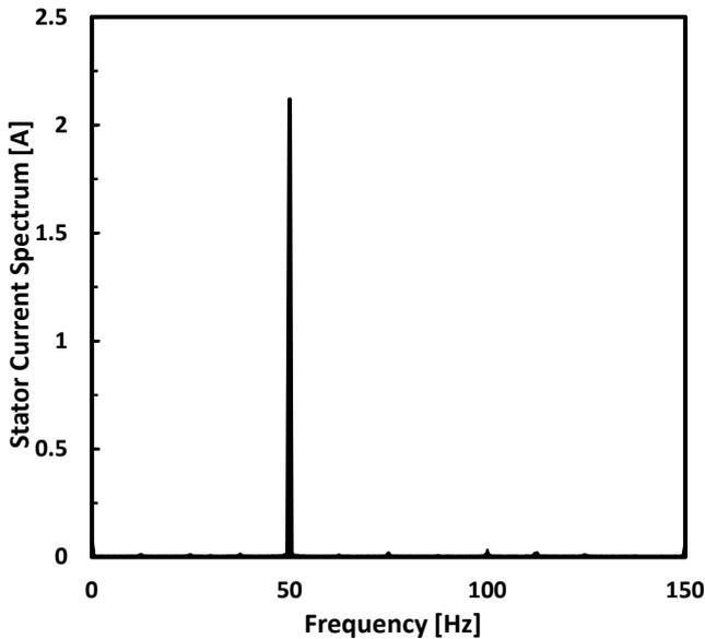
Fig. 6 Amplitude spectrum of the acquired stator current of the machine without rotor eccentricity.
