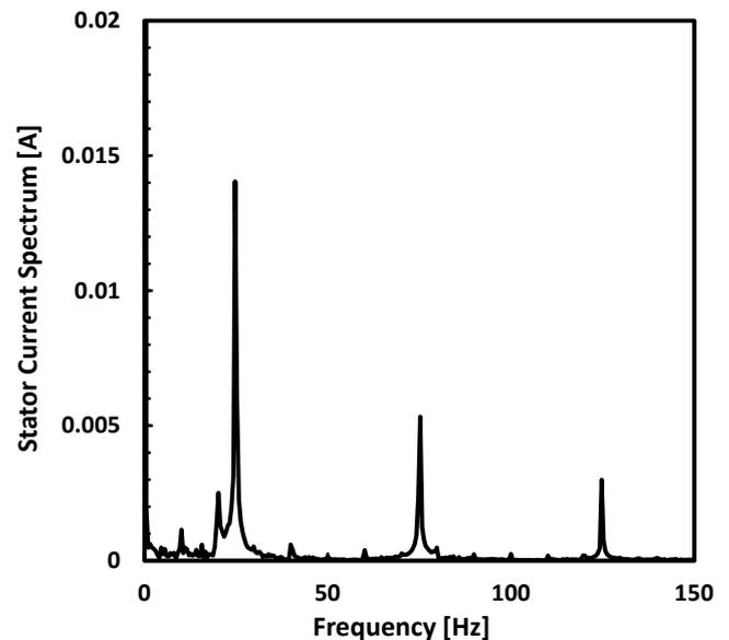
Fig. 11. Amplitude spectrum of RMS value of the stator current the machine with rotor eccentricity.
