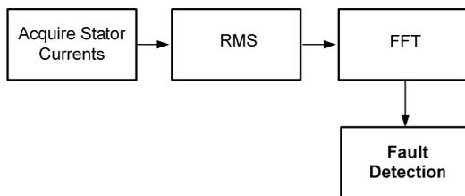
Fig. 1. Method used to detect rotor eccentricity faults.
