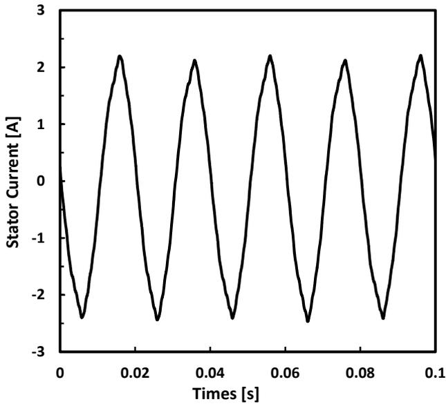
Fig. 5. Experimental stator current of the machine with rotor eccentricity.
