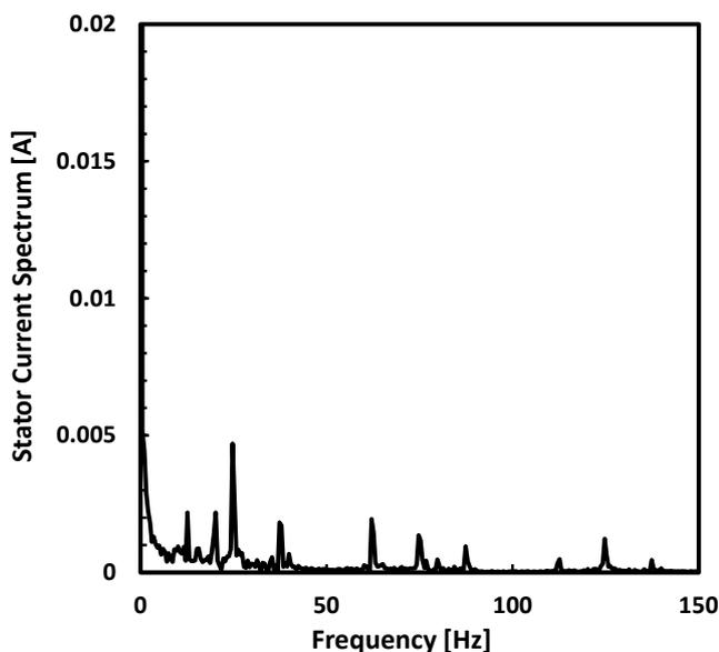
Fig. 10. Amplitude spectrum of RMS value of the stator current the machine without rotor eccentricity.
