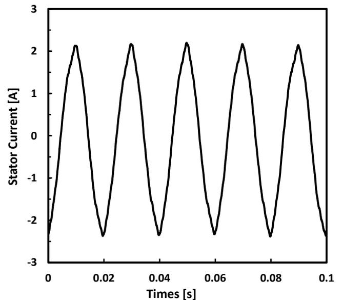
Fig. 4. Experimental stator current of the machine without rotor eccentricity.
