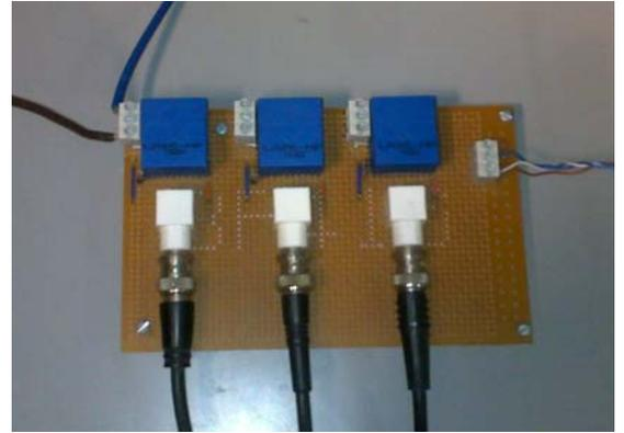
Fig. 3. Stator current measurement sensors.
