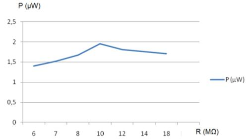
Figure 7: Graph of power in function of load resistance.
