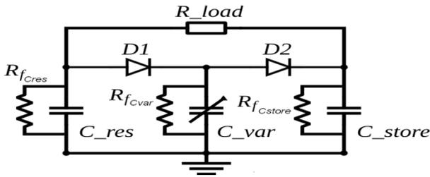
Figure 2. New architecture with the representation of the leakage resistances.
