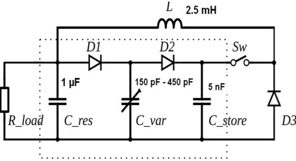
Figure 1. Circuit for energy harvesting.
