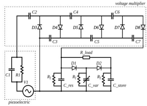
Figure 6: Attachment of the piezoelectric generator to the circuit with variable capacitor.
