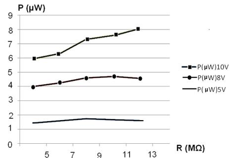
Figure 5: Graph of harvested power for the 5, 8 and 10 V to the proposed architecture.
