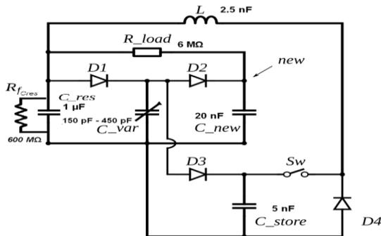
Figure 3. New architecture with flyback.
