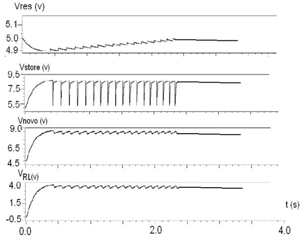
Figure 4. Waveform over  $V_{Cnew}$ ,  $V_{Cstore}$ ,  $V_{Cres}$  and  $V_{RLoad}$ .
