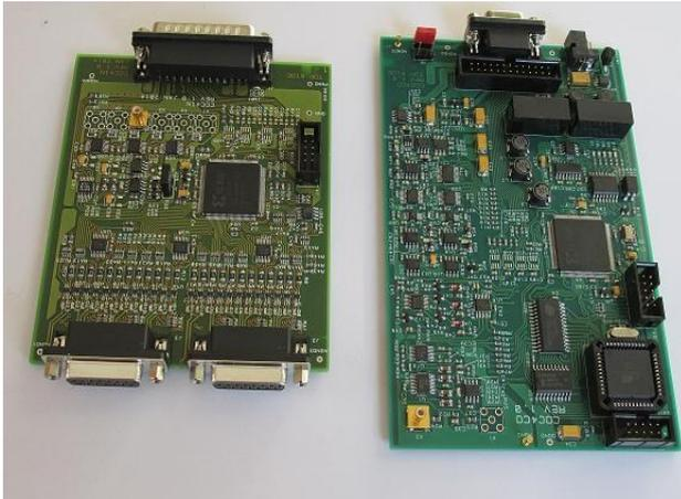
Fig. 3. Assembled boards of the input amplifier (left) and the analog-to-digital converter (right).
