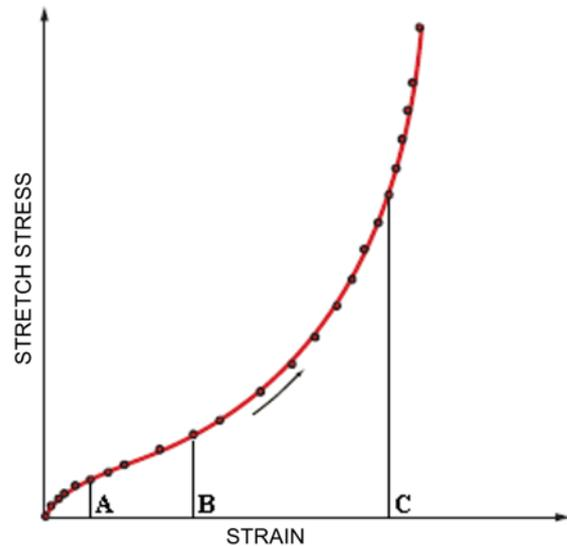
Fig. 5 - Typical stress-strain graph of a vulcanized elastomer
