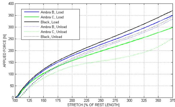
Fig. 10 - Category 19 mm. Test results comparison: despite having the same cross-sections, some compounds suffer a more pronounced elongation factor and stay in traction time
