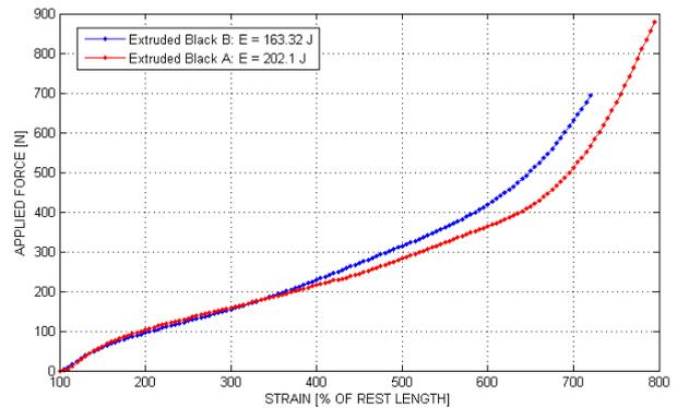
Fig. 13 - Category 16 mm: Elongation until the breakage
