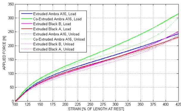
Fig. 11 - Category 16 mm: experimental curves with waiting time of 15 min before unloading
