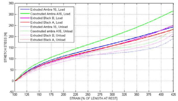
Fig. 12 - Category 16 mm: experimental curves with waiting time of 60 min before unloading
