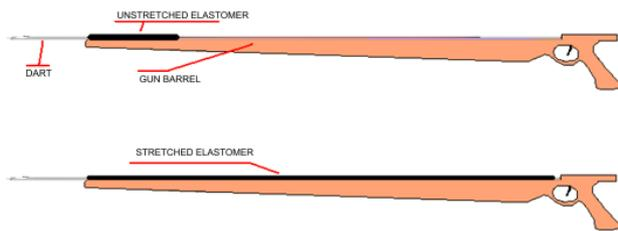
Fig. 1 - Schematic of a speargun and stretching of the elastic phase of armament.
