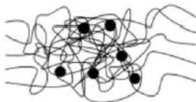
Fig. 3 - Schematic of the elastomeric chains in the undeformed state
