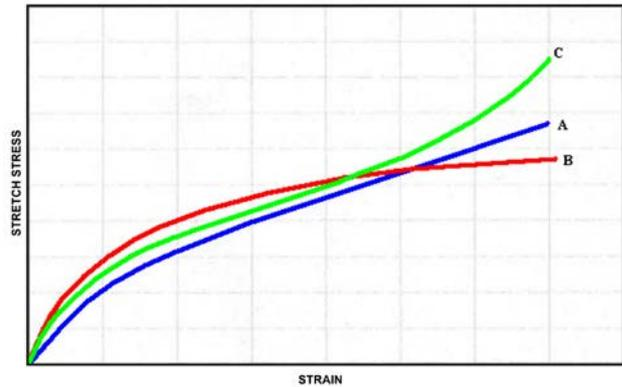
Fig. 6 - Comparison between three types of elastics. The diameters and the rest length are equal.
