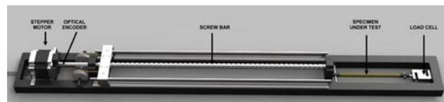
Fig. 7 - Photo of the mechanical section of the test system
