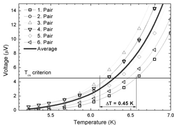
Figure 8. The  $T_{CS}$  measurements from individually post-processed voltage compared with the averaged signal.
