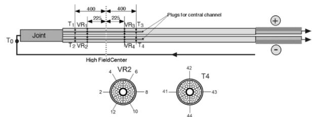
Fig. 6. SULTAN sample voltage and temperature sensor location
