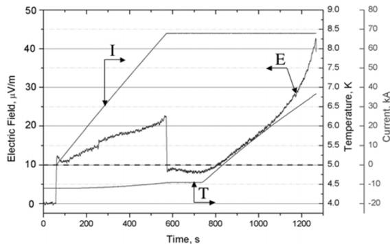
Figure 7. Example of 'voltage slope', i.e. potential building up during the current ramp in a  $T_{CS}$  run.
