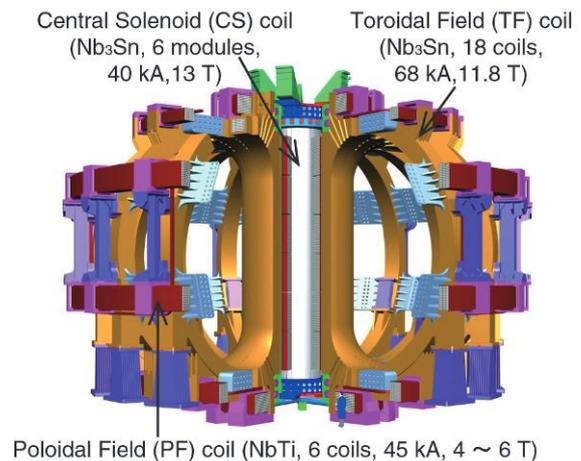
Fig. 1. ITER superconducting magnet system.
