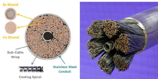
Fig. 2. Views of the ITER TF conductors and of its components [5].
