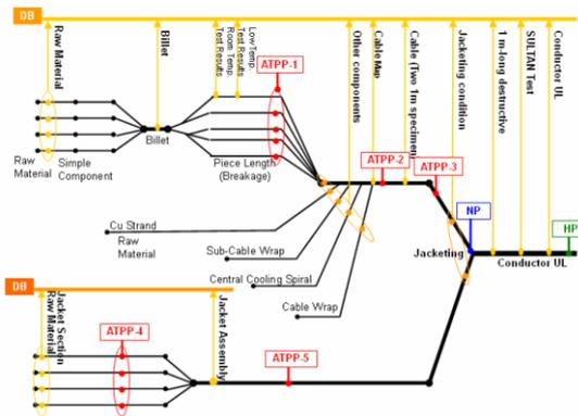
Fig. 4. Control points for monitoring the intermediate assemblies for ITER conductor production [6].
