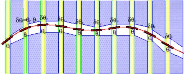
Fig. 5: Schematic view of a volume-track formed by a sequence of base-tracks with their angular measurements in a section of a ECC detector.
