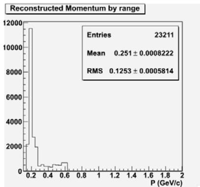
Fig. 11: Distribution of reconstructed momentum by range method considering the signal tracks.
