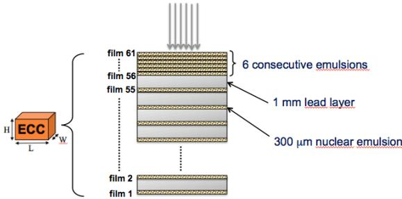
Fig. 2. Details of the ECC structure.
