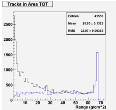
Fig. 8: Distribution of the massive range tracks. The black curve is relative to the signal and the blue one is for the cosmic rays.
