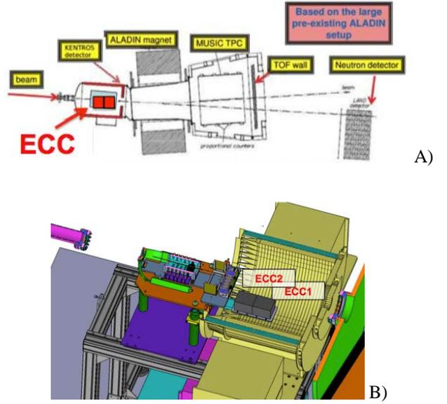
Fig. 3: A) Schematic layout of the FIRST experiment at GSI. The location of two ECC detectors is highlighted; B) Zoomed view of the KENTROS region with the ECC detectors.
