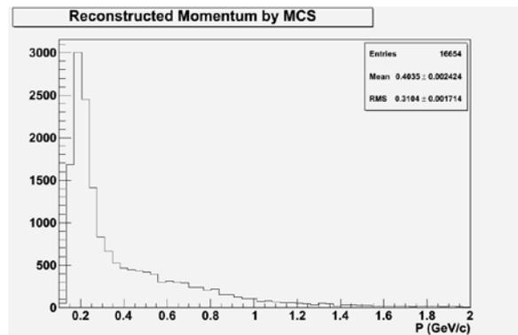
Fig. 10: Distribution of reconstructed momentum by MCS method considering the signal tracks.
