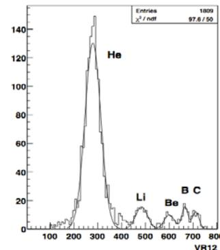
Fig. 1: Charge separation of the fragments generated along the detector by a <sup>12</sup>C ion beam (400 MeV/nucleon).
