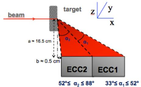
Fig. 4: Layout of the ECC detectors, the  $^{12}\text{C}$  beam and the target; relative distances and the angles with respect to the beam axis are indicated (along  $x$  axis).
