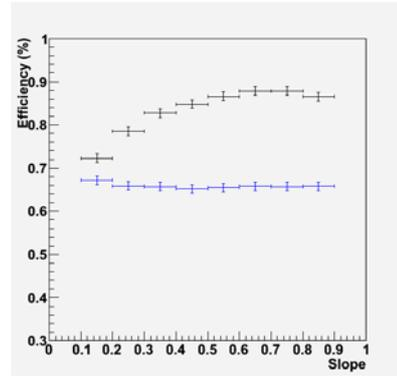
Fig. 9: Track efficiency evaluated on signal (black dots) and on cosmic rays (blue dots) as function of the tracks angle tangent.
