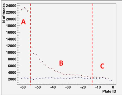
Fig. 7: Number of tracks as a function of film number (plate ID); the signal tracks are plotted in red and the cosmic rays tracks are plotted in blue. The region A, B and C are explained in the text.
