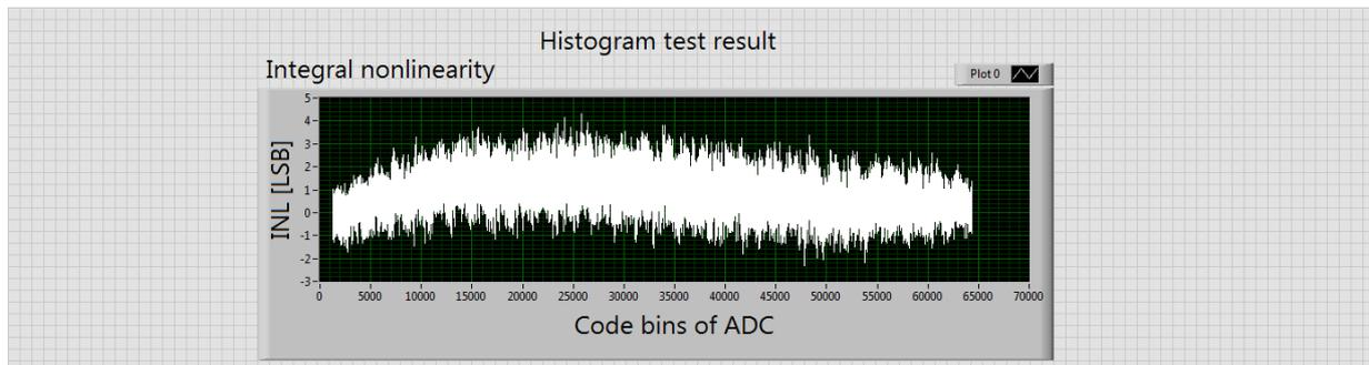
Figure 1. INL characteristics of the tested ADC
