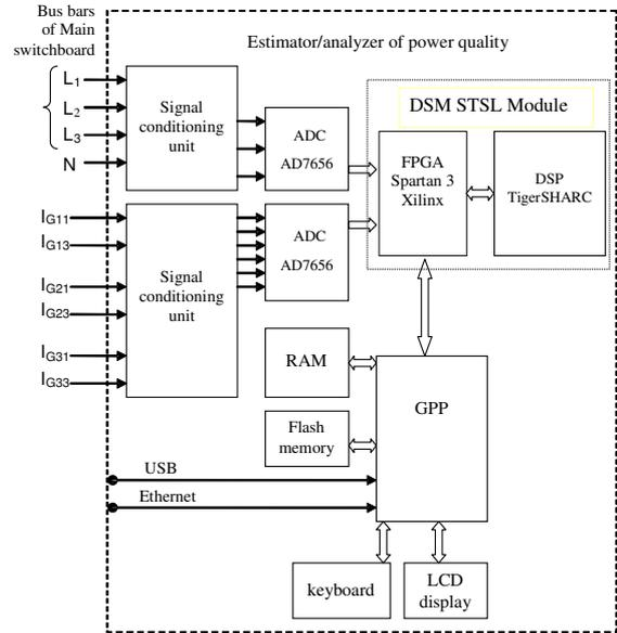
Fig. 3. The hardware structure of instrument [5]
