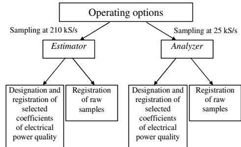
Fig. 4. Main operations performed in instrument
