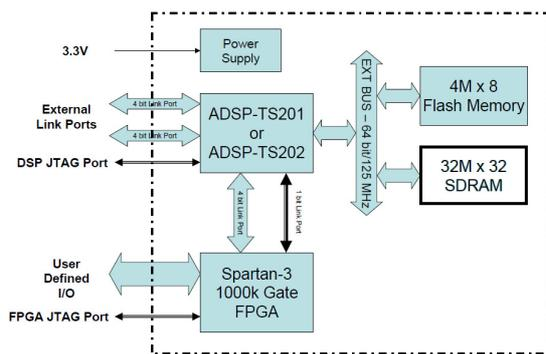
Fig. 8. The block diagram of DSM STSL module [6]
