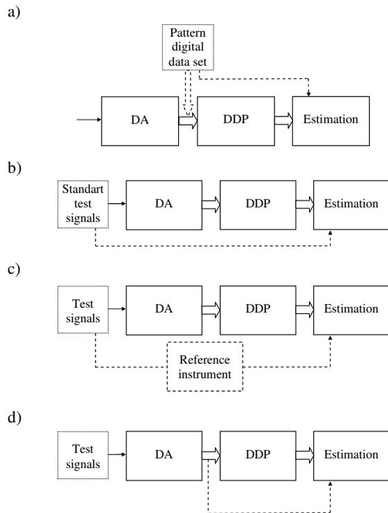
Fig. 2. The exemplary layouts for calibration of digital channel for measurement of analogue quantity : a) using pattern digital data set, b) using standart analogue test signals, c) with reference system, d) using collected digital data
