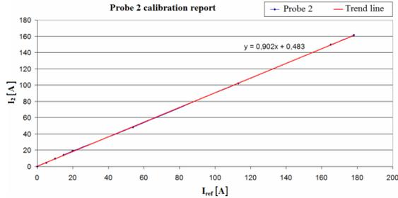
Fig. 5. The exemplary calibration report of current probe No. 2
